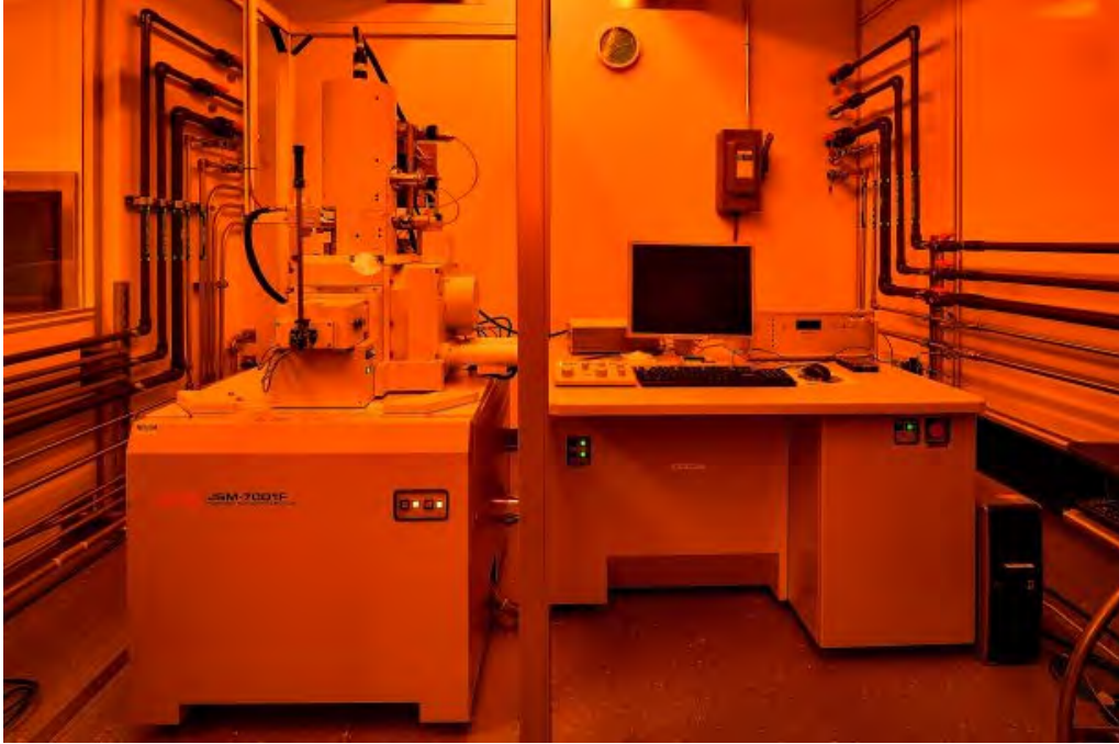
FIGURE 3.12. Shows the JEOL JSM-7001F SEM at the MRF. The SEM is on the left-hand side of the image. The XENOS XPG2 e-beam pattern writer is at the right-hand side of the image, seated on the table.
