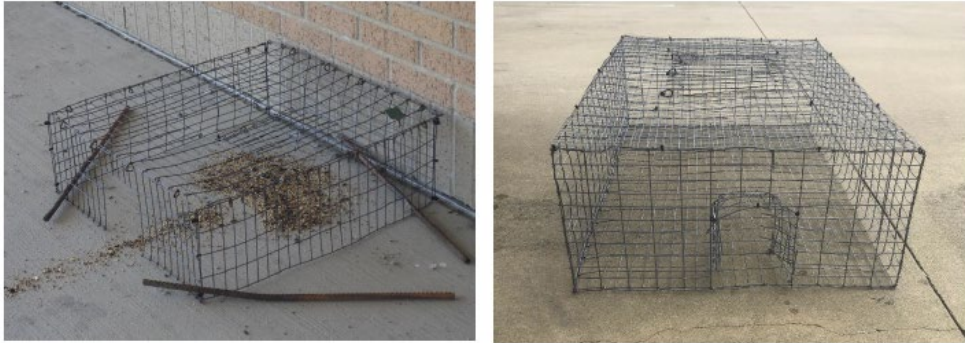
Figure 2.7: Left, a baited open trap with the funnel removed and the top access door open. Right, a similar trap with the funnel attached and top access door secured.
