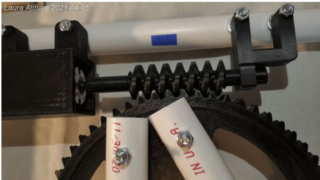
Figure 5.1: Worm gear assembly testing.
