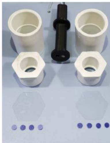
Figure 4.2: Sensor holder assembly and components.
