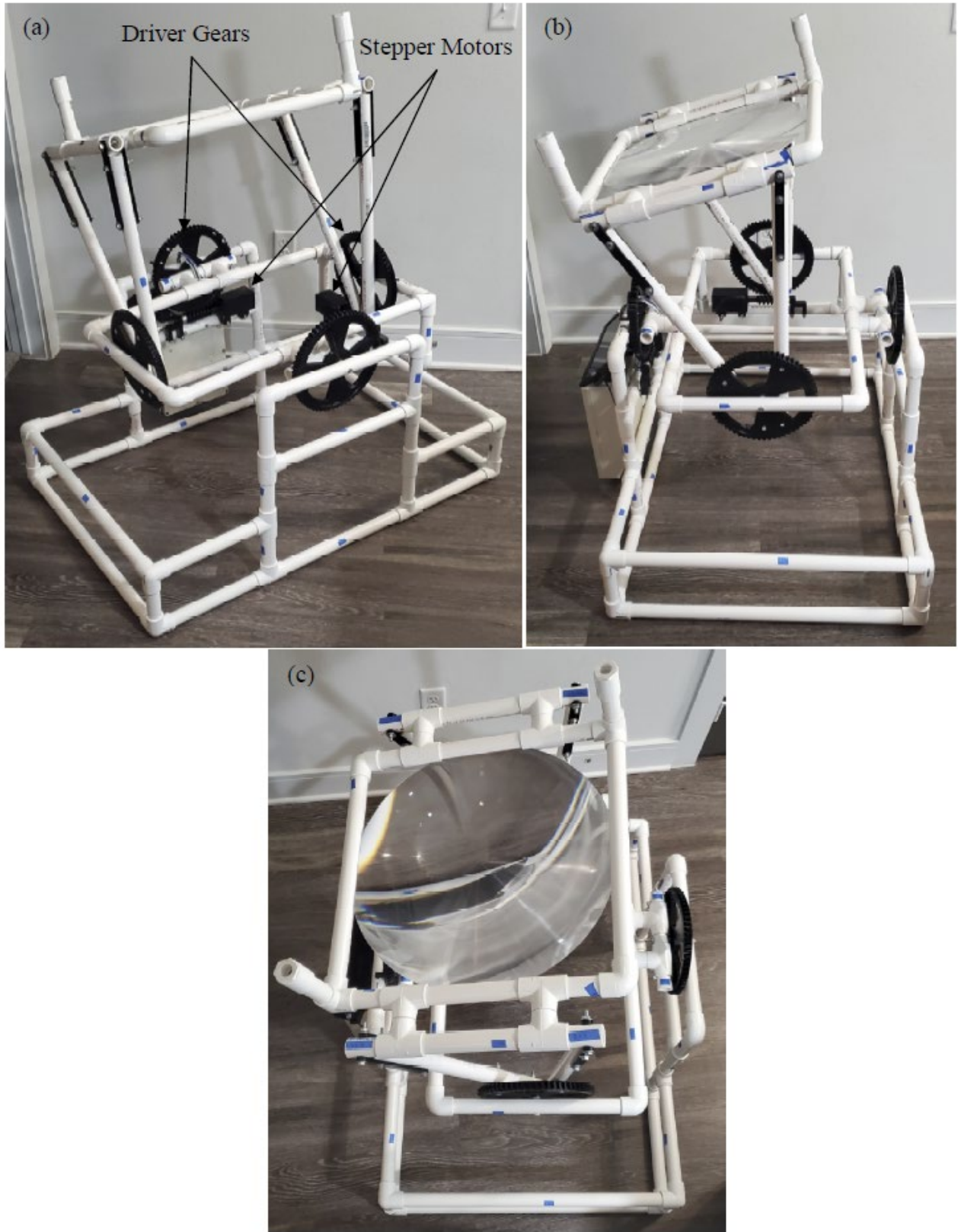
Figure 3.5: (a) – (c) Different perspectives of the solar tracker project.
