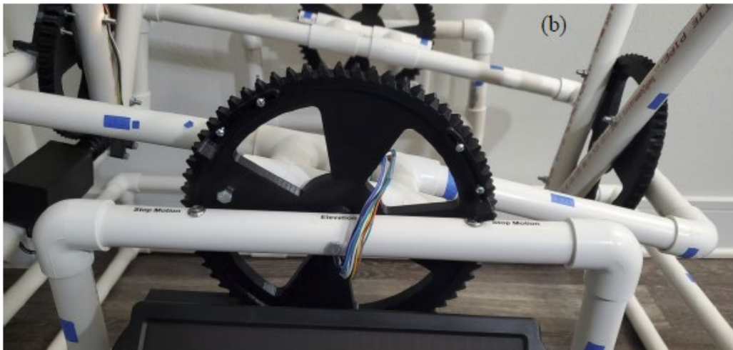
Figure 5.4: Testing of (a) manual positioning switches, and (b) switches of stopping motion and the right side stopper motion pad.
