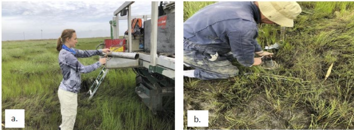
Figure 3.2: (a) Sawing off excess core tube in the marsh to the south of Clam Lake. (b) Placing a vacuum seal into a core tube prior to retrieval.
