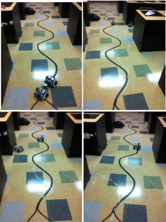
Fig. 10: In the picture shown, a slightly different track involving both left and right turns. UL: Shows the starting positions for the lead and follow robots for each trial. The lead robot traced the black line while the white line represents the movement of the follower robot.
