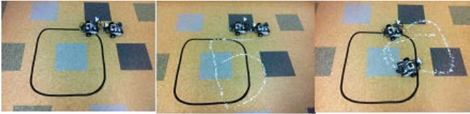
Fig. 9: Left: Shows where the two robots started and each picture involves a complete circle by the lead robot. The lead robot faithfully followed the box in a counterclockwise direction while the follow robot received the Bluetooth information. The lead robot traced the black line while the white line represents the movement of the follow robot.
