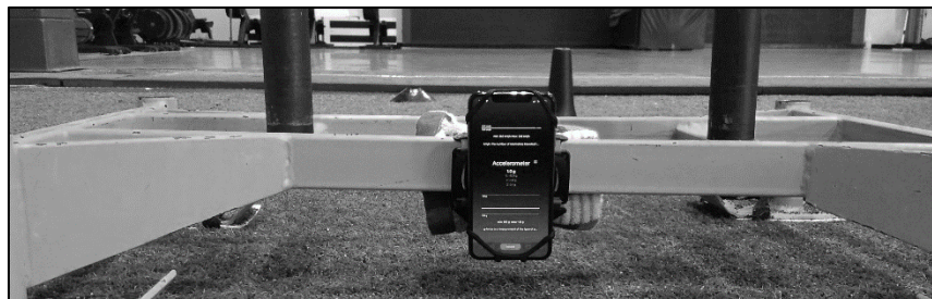
Figure 2.2: iPhone accelerometer placement.
