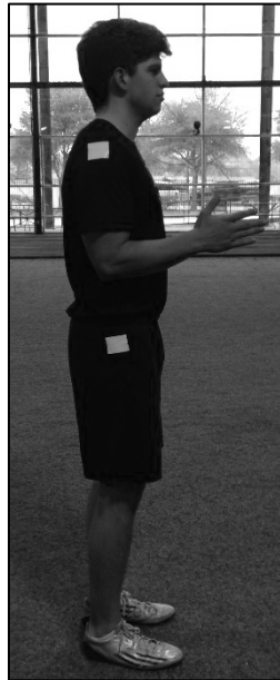
Figure 2.4: Joint markers (greater tuberosity (shoulder) and greater trochanter (hip)).
