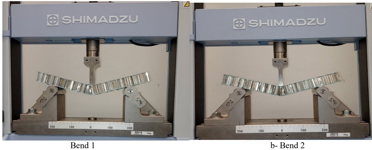
Figure 5.23: Mechanical test of the 3-point bend
