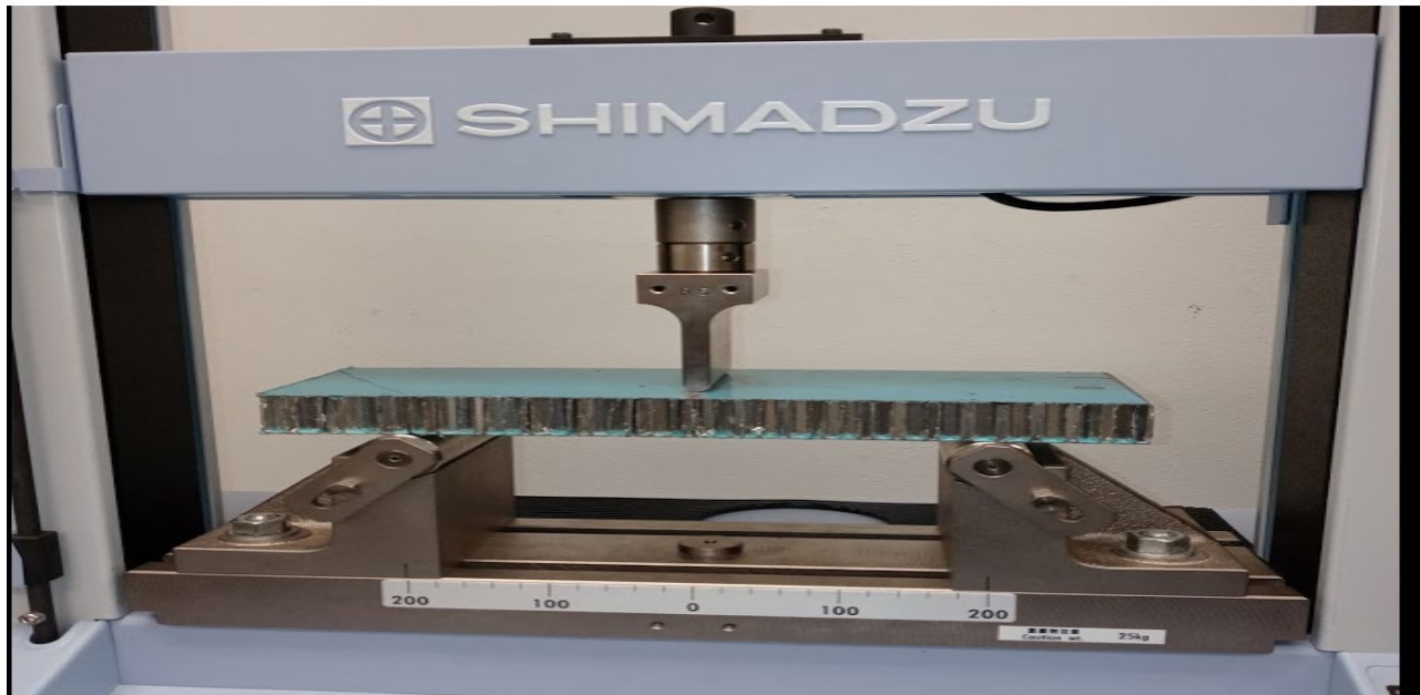
Figure 4.8: Test fixture on test resource machine for the three-point bend
