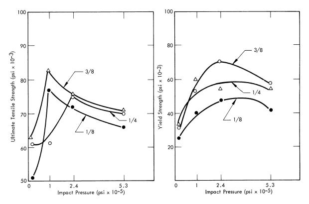
Figure 15. EFFECT OF AMBIENT-TEMPERATURE IMPACT ON THE TENSILE PROPERTIES OF CAST URANIUM. (1/8, 1/4, and 3/8-Inch Thick)
