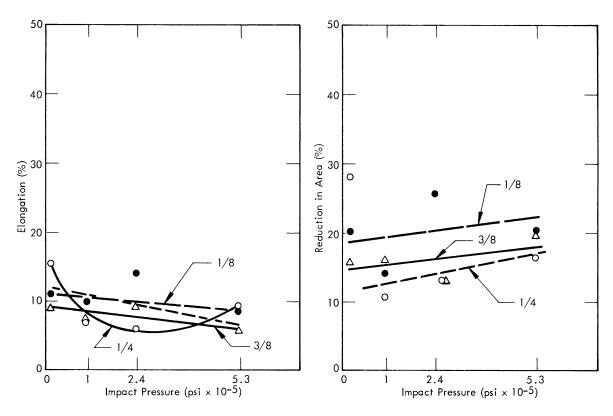
Figure 18. EFFECT OF  $37.5^{\circ}$  F IMPACT AND VACUUM HEAT TREATMENT ON THE DUCTILITY OF CAST URANIUM. (1/8, 1/4, and 3/8-Inch Thick)
