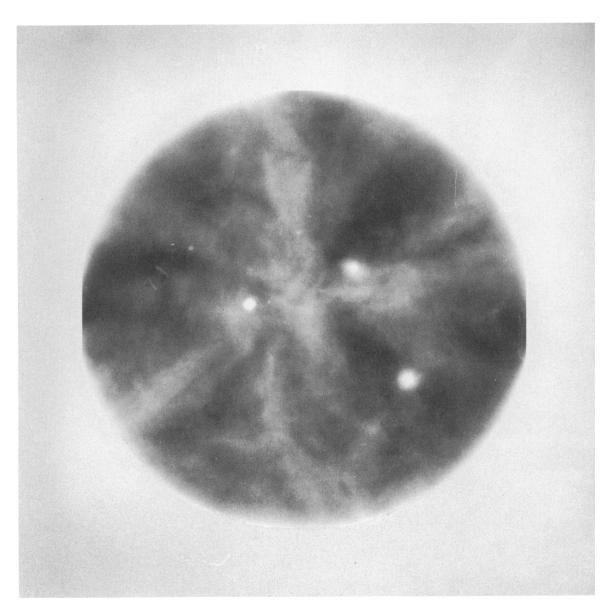
Figure C-14. DISC 712 AFTER  $375^{\circ}$  F IMPACTION AT 2.4 X  $10^{5}$  PSI.
