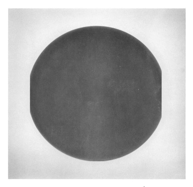
Figure C-6. DISC 502 AFTER  $375^{\circ}$  F IMPACTION AT 2.4 X  $10^{5}$  PSI.
