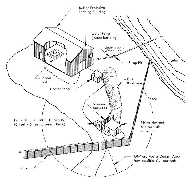
Figure A-5. TASK I, II, & IV - TEST FACILITY FOR EXPLOSIVE CONDITIONING AND COMPACTION.
