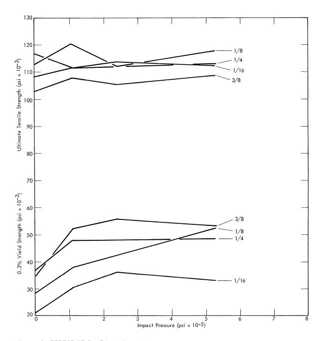
Figure 12. EFFECT OF 375°F IMPACT AND VACUUM HEAT TREATMENT ON THE TENSILE PROPERTIES OF WROUGHT URANIUM. (Data Taken from Tables 4 and 6)
