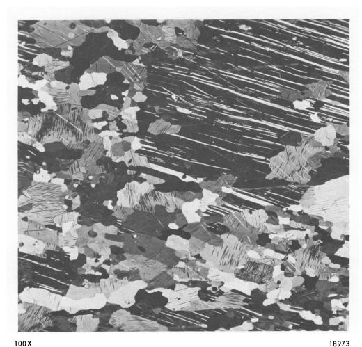
Figure 24. MICROSTRUCTURE OF A 1/8-INCH WARM IMPACTED AND ANNEALED CAST URANIUM DISC. (Estimated Impact Pressure  $-5.3 \times 10^5$  psi; Cross-Section View)
