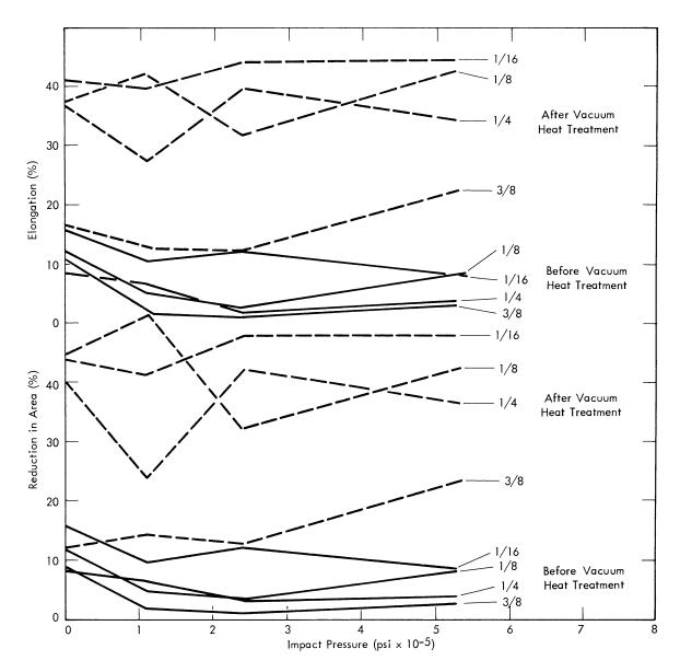
Figure 13. EFFECT OF AMBIENT-TEMPERATURE IMPACT ON THE DUCTILITY OF WROUGHT URANIUM. (Data Taken from Tables 4 and 5)
