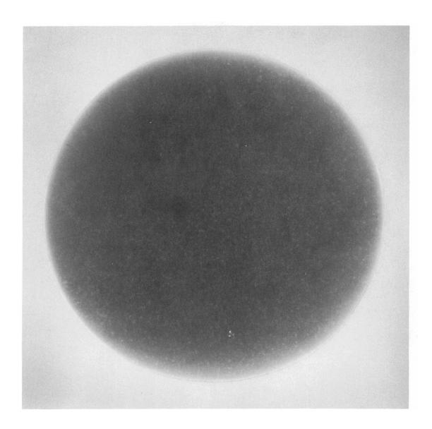
Figure C-3. DISC 304 (1/4-INCH THICK) ROLLED AND SALT ANNEALED; NOT IMPACTED.
