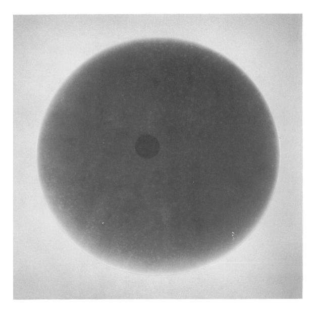
Figure C-1. DISC 301 (1/4-INCH THICK) ROLLED AND SALT ANNEALED; NOT IMPACTED. (Large Marking is a Penetrameter)
