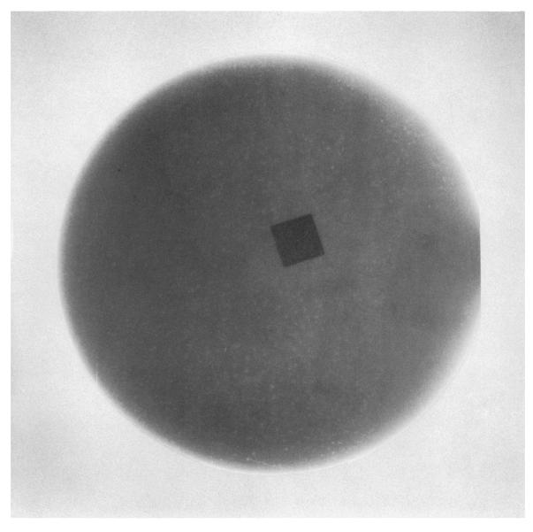
Figure C-2. DISC 301 AFTER AMBIENT-TEMPERATURE IMPACTION AT 1.1 X  $10^5$  PSI. (Large Marking is a Penetrameter)
