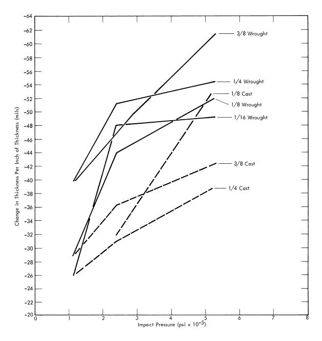
Figure 6. RELATIVE CHANGE IN URANIUM THICKNESS WHEN IMPACTED AT  $375^{\circ}$  F. (Data Taken from Table 3)
