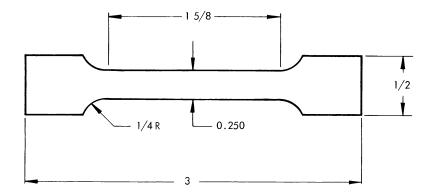
Figure 8. THREE-INCH FLAT TENSILE SPECIMEN. (Thickness - 0.100 lnch)
