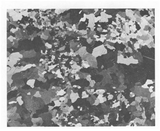
$100 \, \text{X}$  Figure 23. MICROSTRUCTURE OF A 1/8-INCH WARM IMPACTED AND ANNEALED CAST URANIUM DISC. (Estimated Impact Pressure  $-5.3 \times 10^5$  psi; Surface View)
