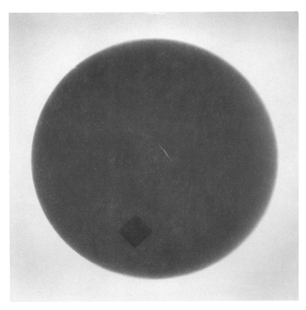
Figure C-4. DISC 304 AFTER AMBIENT-TEMPERATURE IMPACTION AT 1.1 X  $10^5\,$  PSI.
