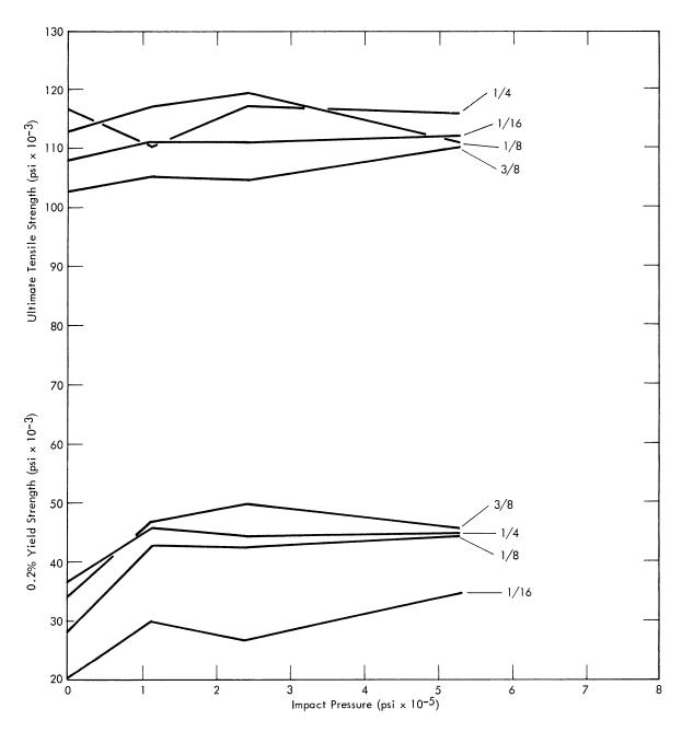
Figure 11. EFFECT OF AMBIENT-TEMPERATURE IMPACT AND VACUUM HEAT TREATMENT ON THE TENSILE PROPERTIES OF WROUGHT URANIUM. (Data Taken from Tables 4 and 5)
