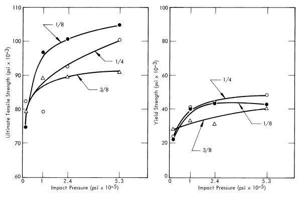
Figure 17. EFFECT OF 375°F IMPACT AND VACUUM HEAT TREATMENT ON THE TENSILE PROPERTIES OF CAST URANIUM. (1/8, 1/4, and 3/8-Inch Thick)
