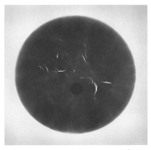
Figure C-10. DISC 313 AFTER AMBIENT-TEMPERATURE IMPACTION AT 5.3 X  $10^5\,$  PSI.
