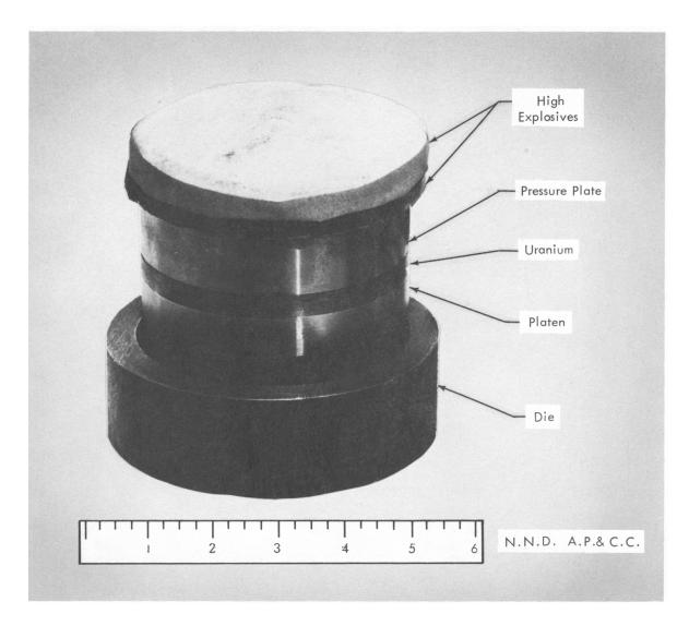
Figure A-4. TEST COMPONENTS ASSEMBLED IN SEQUENCE.
