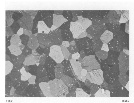
Figure 19. MICROSTRUCTURE OF A 3/8-INCH SALT-ANNEALED WROUGHT URANIUM DISC. (Not Impacted)
