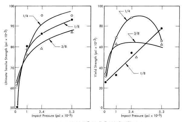
Figure 16. EFFECT OF 375°F IMPACT ON THE TENSILE PROPERTIES OF CAST URANIUM. (1/8, 1/4, and 3/8-Inch Thick)
