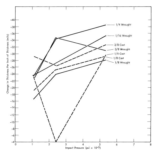
Figure 5. RELATIVE CHANGE IN URANIUM THICKNESS WHEN IMPACTED AT AMBIENT TEM-PERATURE. (Data Taken from Table 3)
