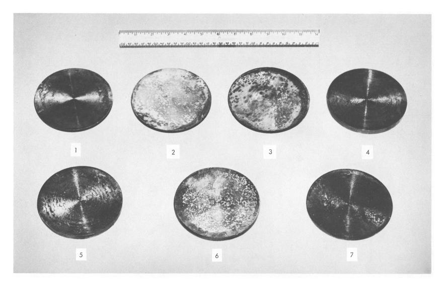
Figure B-1. BERYLLIUM-COPPER DISCS AFTER TEST.
