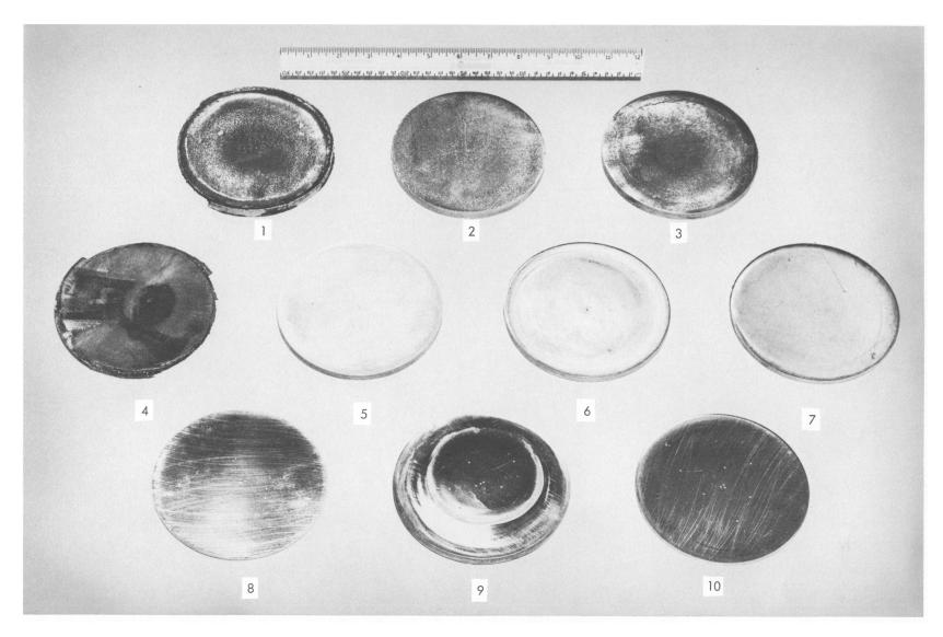
Figure A-6. TYPE 430 STAINLESS STEEL DISCS AFTER TEST.
