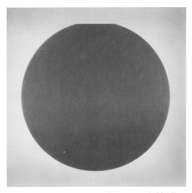
Figure C-5. DISC 502 (1/16-INCH THICK) ROLLED AND SALT ANNEALED; NOT IMPACTED.
