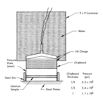
Figure A-2. TASK I & II - CONDITIONING URANIUM DISCS. (Test Setup)
