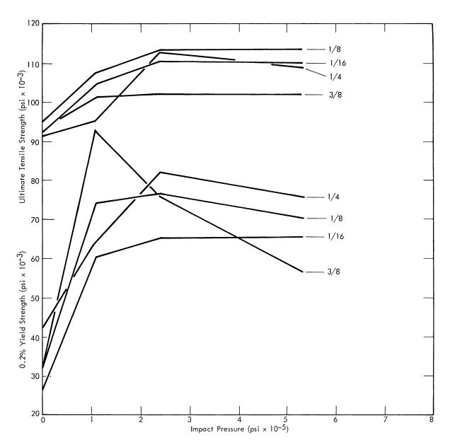
Figure 9. EFFECT OF AMBIENT-TEMPERATURE IMPACT ON THE TENSILE PROPERTIES OF WROUGHT URANIUM. (Data Taken from Tables 4 and 5)
