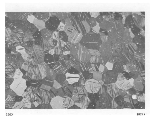
Figure 20. MICROSTRUCTURE OF A 3/8-INCH COLD IMPACTED WROUGHT URANIUM DISC. (Estimated Impact Pressure  $-5.3\times10^5$  psi)
