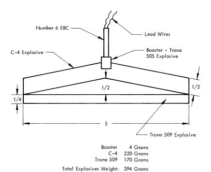
Figure A-1. TASK I & II - CONDITIONING URANIUM DISCS. (Expolsive Charge Geometry)
