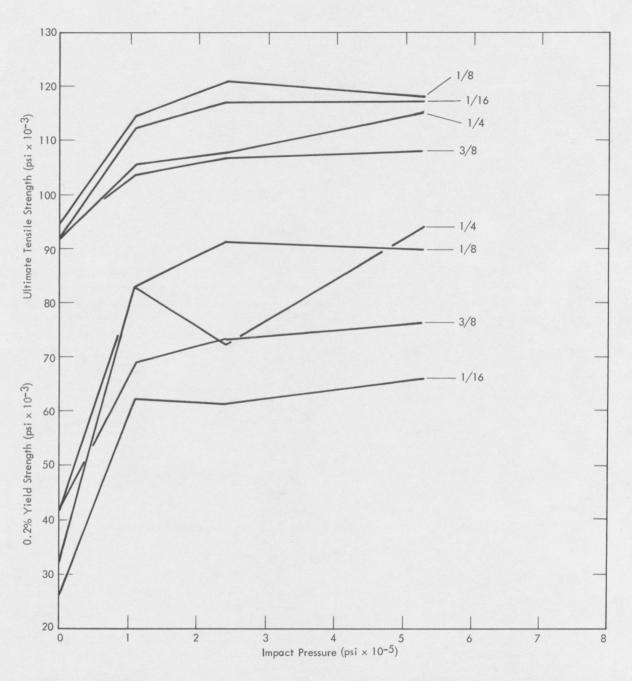
Figure 10. EFFECT OF 375°F IMPACT ON THE TENSILE PROPERTIES OF WROUGHT URANIUM. (Data Taken from Tables 4 and 5)
