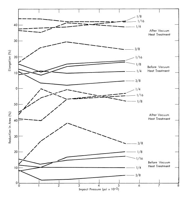
Figure 14. EFFECT OF 375°F IMPACT ON THE DUCTILITY OF WROUGHT URANIUM. (Data Taken from Tables 4 and 6)
