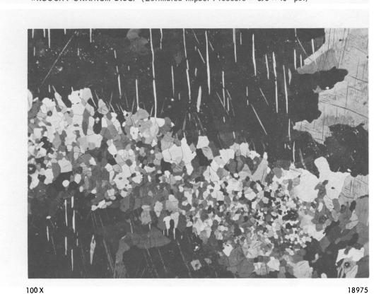
Figure 22. MICROSTRUCTURE OF A 3/8-INCH WARM IMPACTED AND ANNEALED CAST URANIUM DISC. (Estimated Impact Pressure  $-5.3 \times 10^5$  psi; End View)
