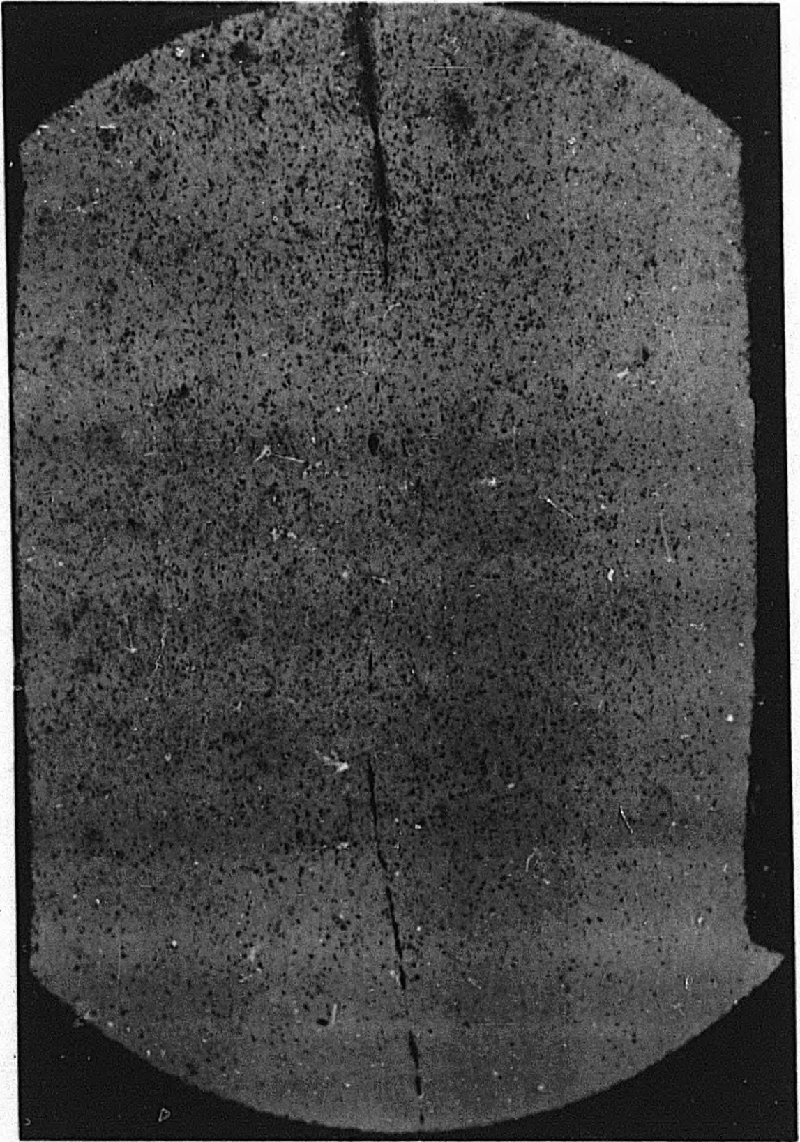
Fig. 4—Microphotograph of cold-welded aluminum.
