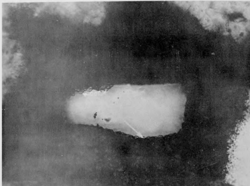
Figure 33. Translucent properties of coffinite (cof)? Same field as figure 32 with transmitted light, 1500 X
