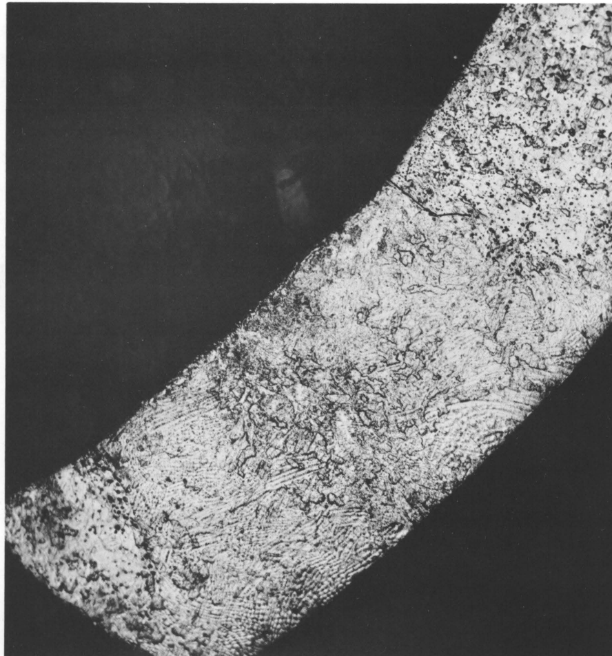
Figure 50. Crack Detected in 406 SS Welded Tubing by an Ultrasonic Technique
