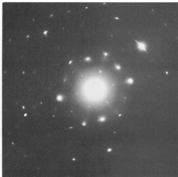
Figure 193. SAD from [111]-Zone Corresponding to Figure 192
