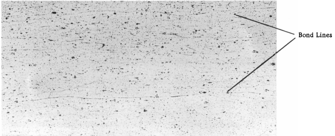
Figure 52. Longitudinal Sections through the 406 Stainless Steel End Cladding of a Depleted Superheat Fuel Plate Showing Bond-line Inclusions
