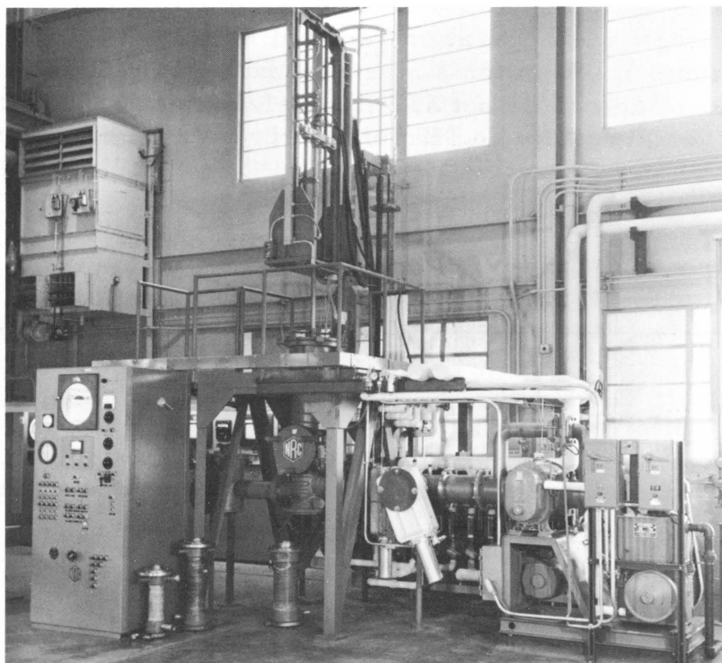
Figure 119. NRC Model 2721A Vacuum Arc Furnace
