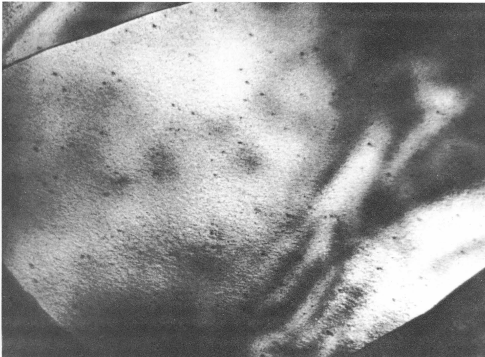
Figure 234 Transmission Electron Photomicrograph of Uranium in the An- nealed Condition
