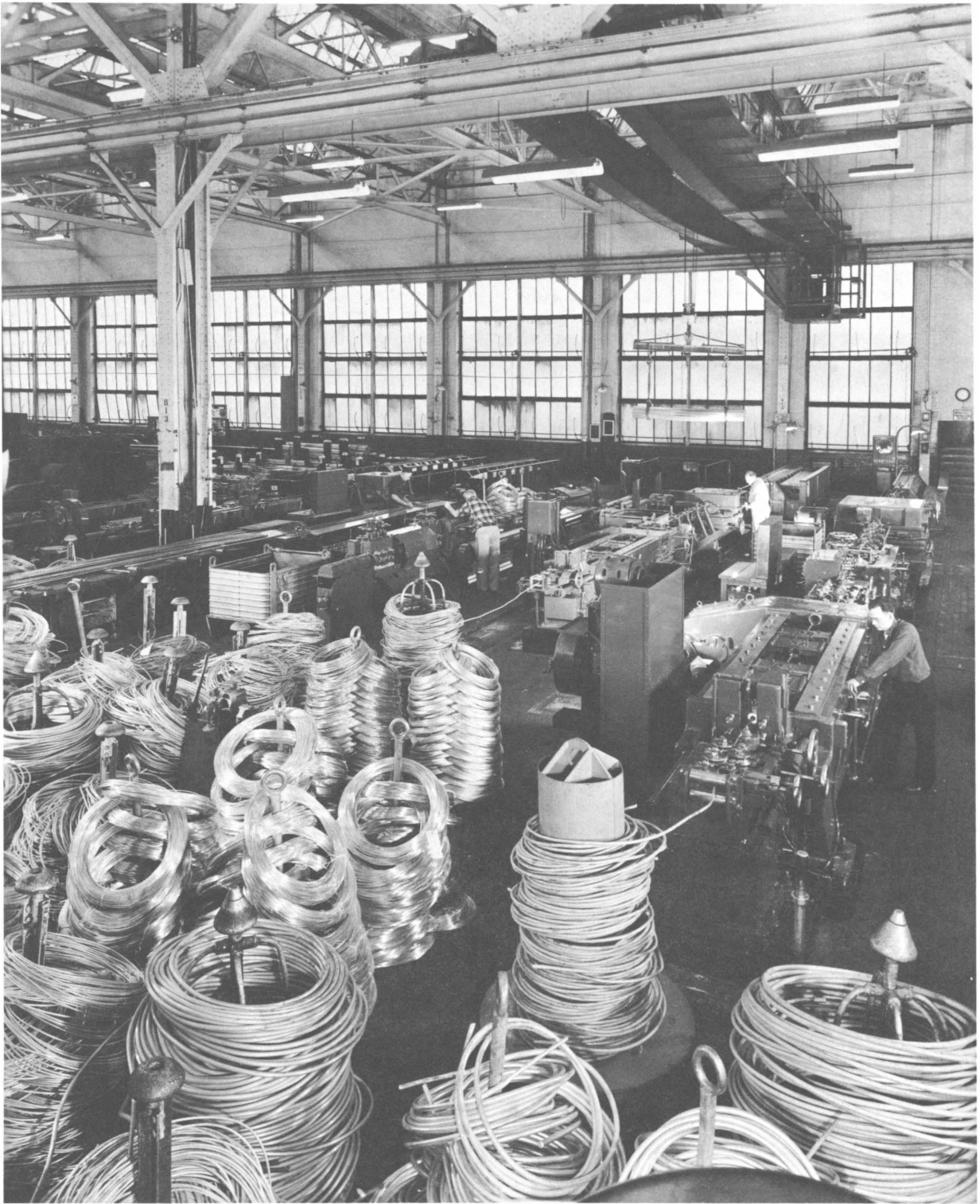
FIGURE 29. —Automatic Rod Drawing, Finishing, and Cutting Machines. (Courtesy, Anaconda American Brass Co.)
