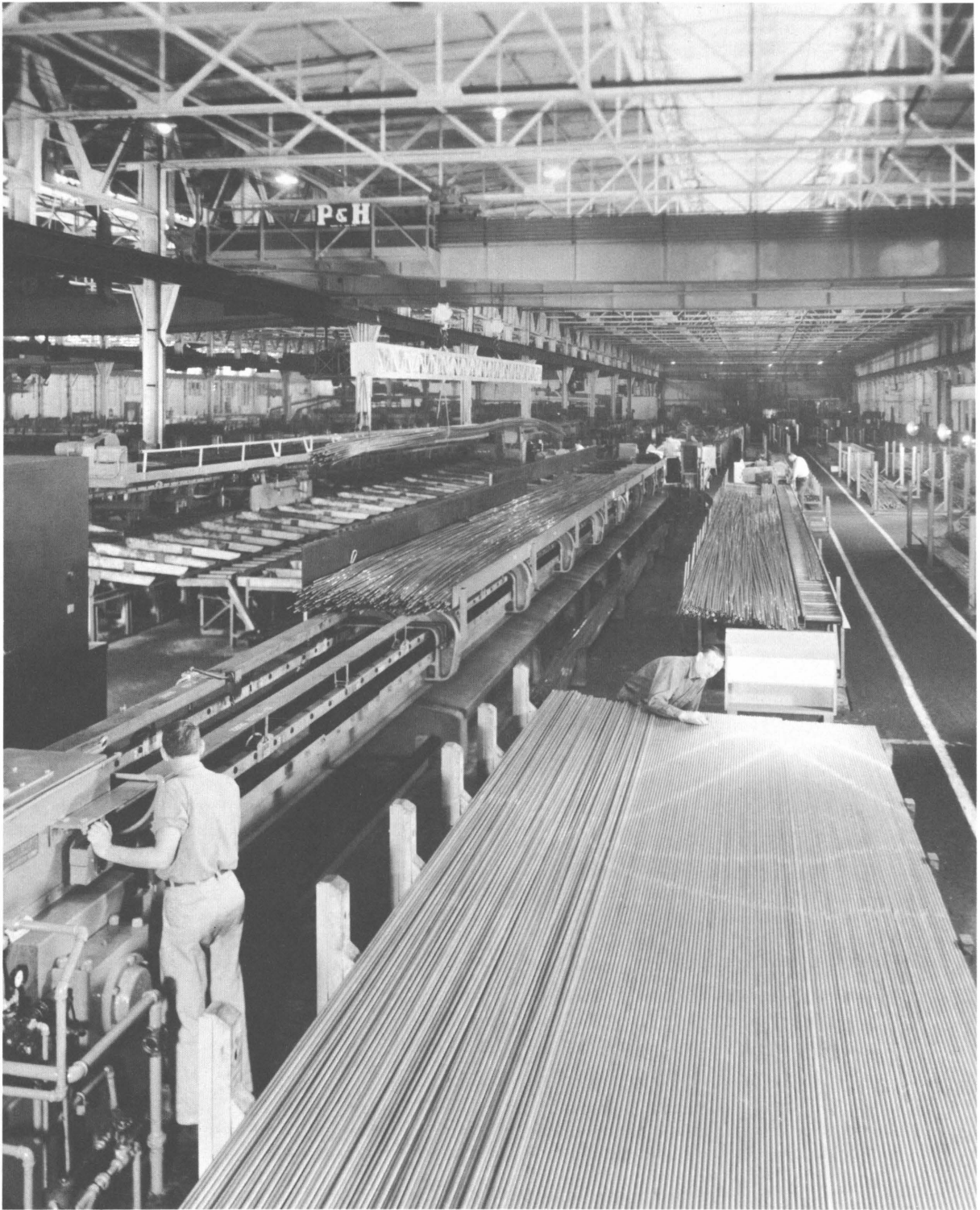
FIGURE 27.—Draw Bench. (Courtesy, Anaconda American Brass Co.)
