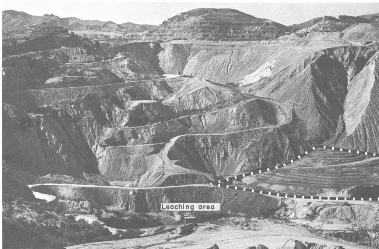
FIGURE 25. - Miami Unit Caved Area, Presently Being Leached by Miami Copper Co., Miami, Ariz.
