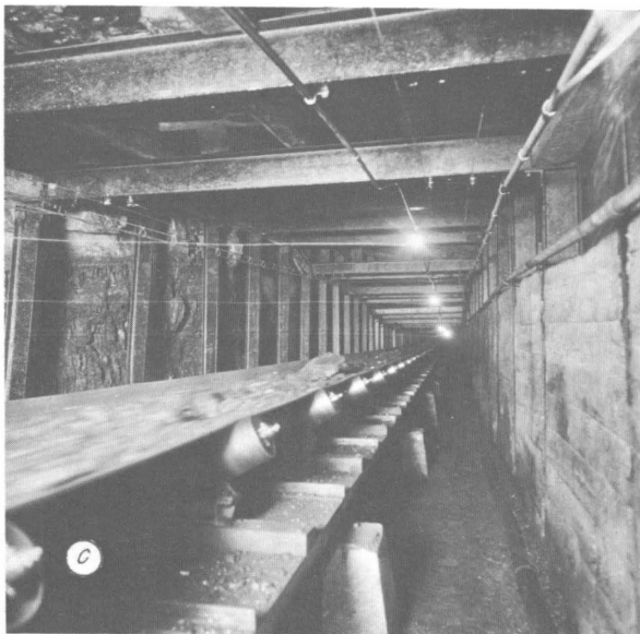
FIGURE 39.—Underground Transportation: A, Mine Train Loading at Chute; B, Truck; C, Conveyor; D, Ore Skips for Hoisting.
