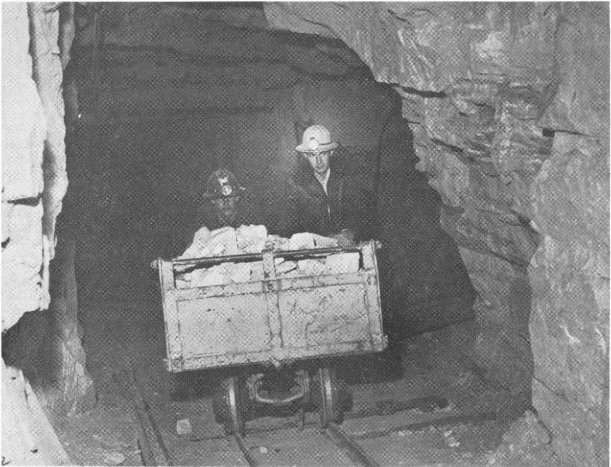
FIGURE 5.—Typical Interior View of Uranium-Vanadium Mine, Showing Rock Wall and Hand-Operated Ore Car.
