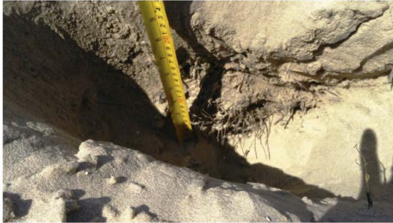
Figure 3.2: Distinct contact between marsh and washover sedimentation.
