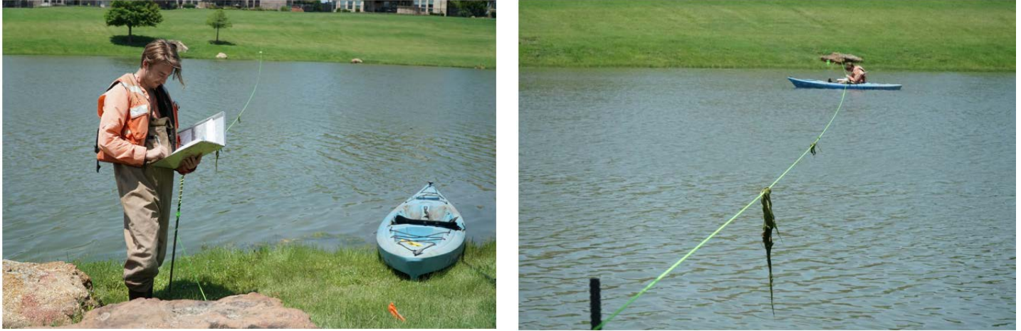
Figure 4.4: Depth survey of LSR-1. (Photos courtesy of Duong Nguyen.)
