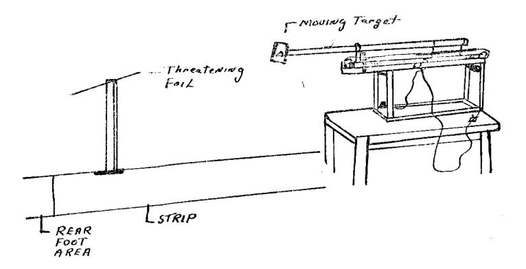
Fig. 1--Mechanical fencing apparatus (Patent Number Pending)
