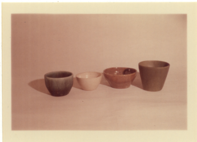
Fig. 4.--Specimens of glazes A , B , C , and D (left to right), on clay body No. 11.
