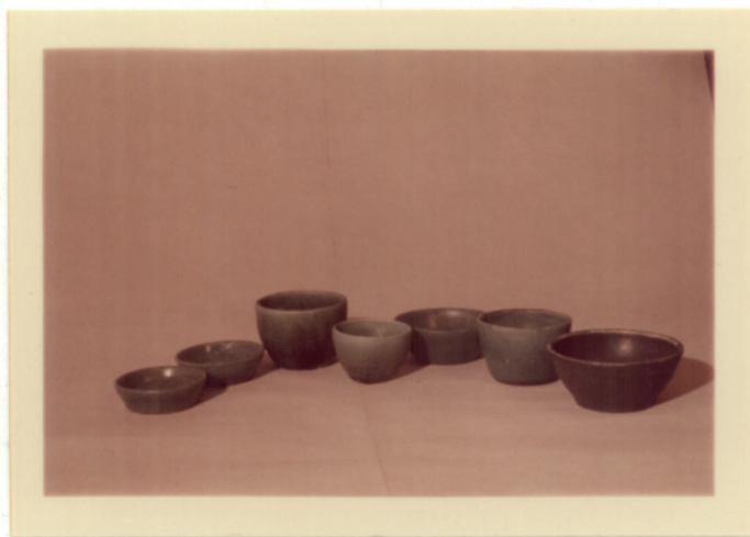
Fig. 7--Specimens of glaze A on clay bodies Nos. 9, 10, 11, 12, 13, 14, and 15 (left to right).
