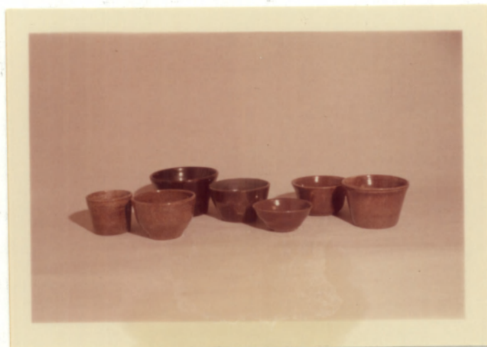
Fig. 9.--Specimens of glaze C on clay bodies No. 2, 3, 7, 8, 13, 14, and 15 (left to right).
