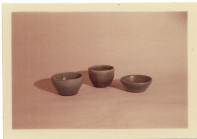
Fig. 5.--Specimens of Glaze A on clay bodies Nos. 2, 13, and 11 (left to right).
