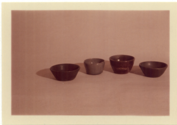
Fig. 3.--Specimens of glazes A , B , C , and D (left to right), on clay body No. 8.
