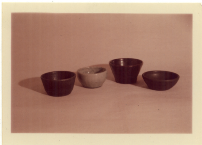
Fig. 2.--Specimens of glazes A , B , C , and D (left to right), on clay body No. 7.
