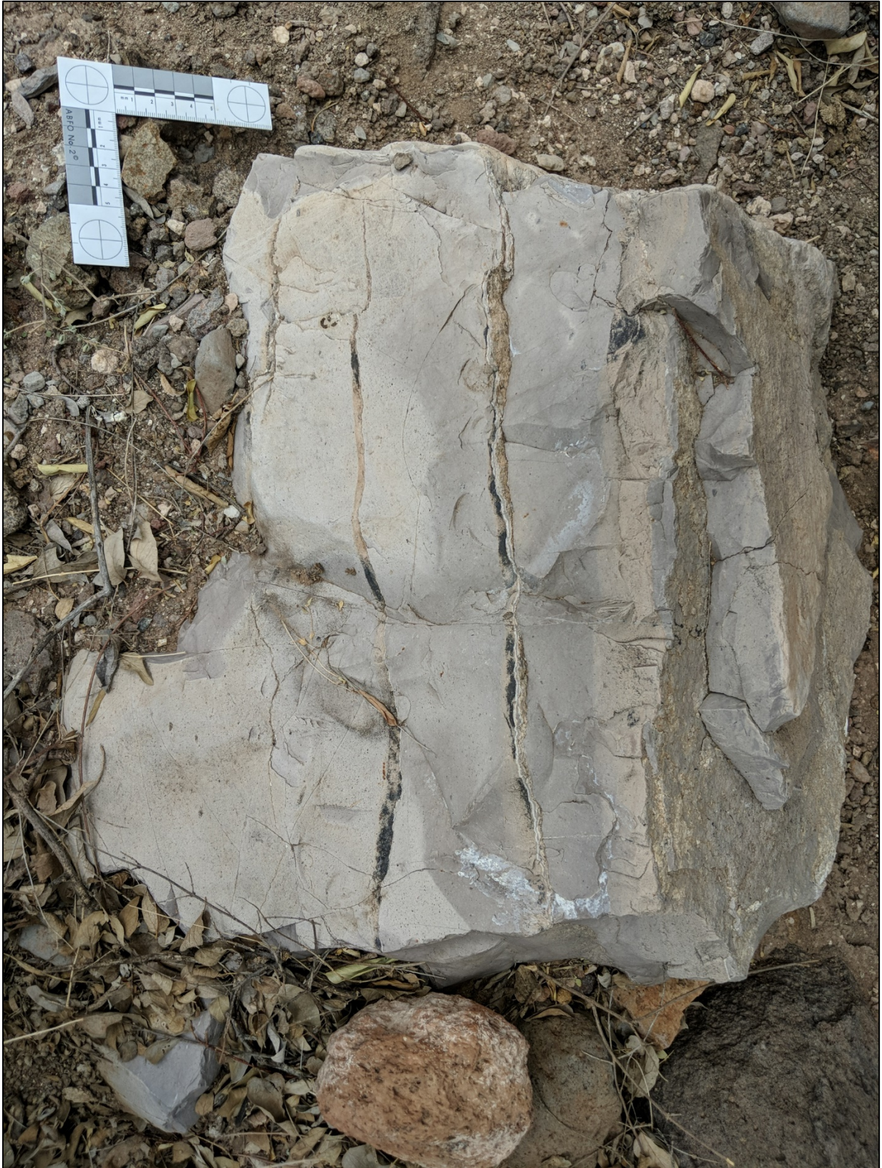
Figure 4.4: Photo of a tuff boulder with chalcedony veins located along Placitas Arroyo channel.
