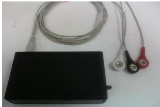
Figure 3.4 - Fully Constructed Enclosure
