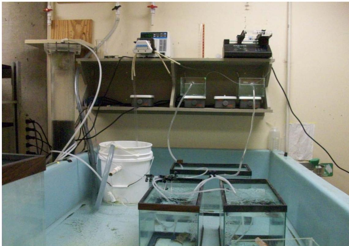
Figure 3. A continuous fish flow-through exposure system used for exposure tests.
