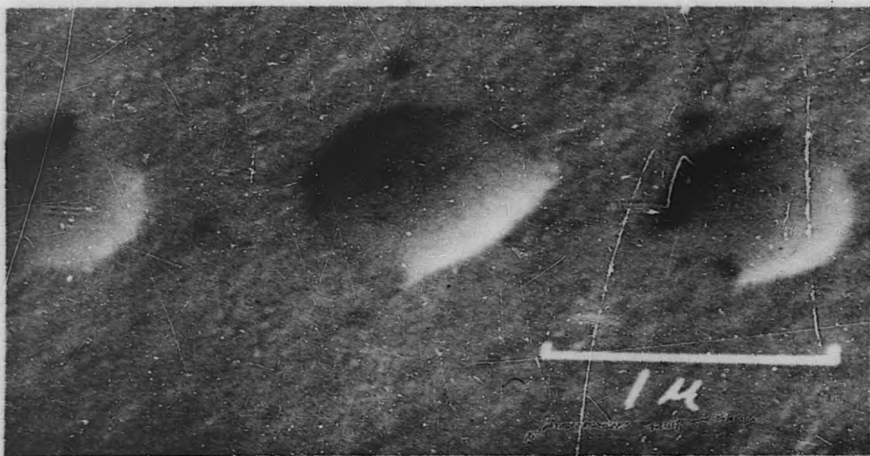
Figure 5. Electron photomicrograph of several immiscible regions in RX70 bead formed under standard conditions.
