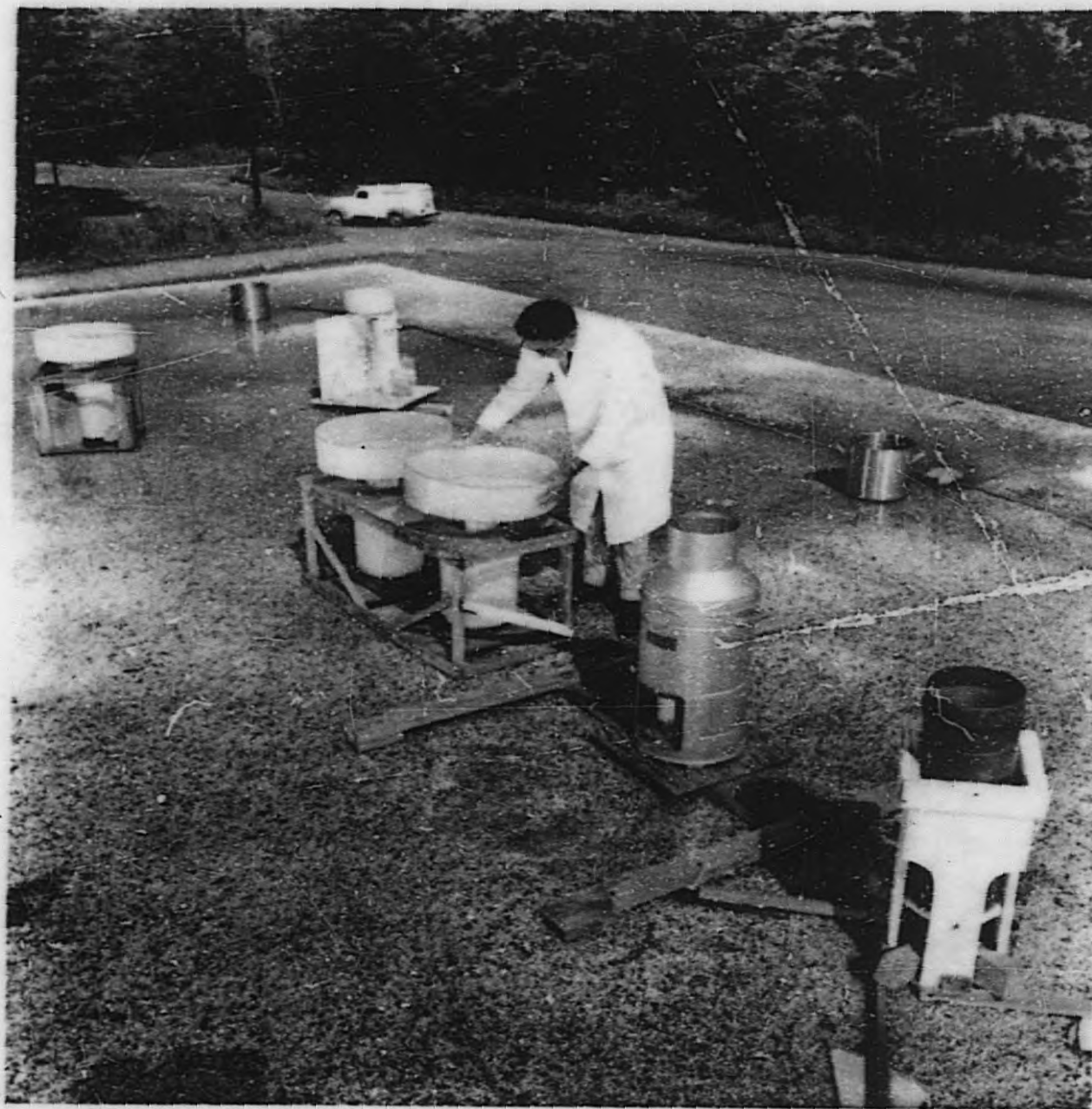
Figure 1. Array of Rain Collection Devices on the Roof at Isotopes, Inc.
