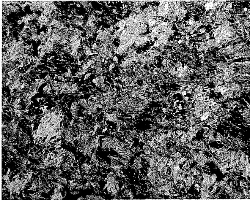
Figure 5-20. Optical micrographs of Stackpole 2020 graphite.
