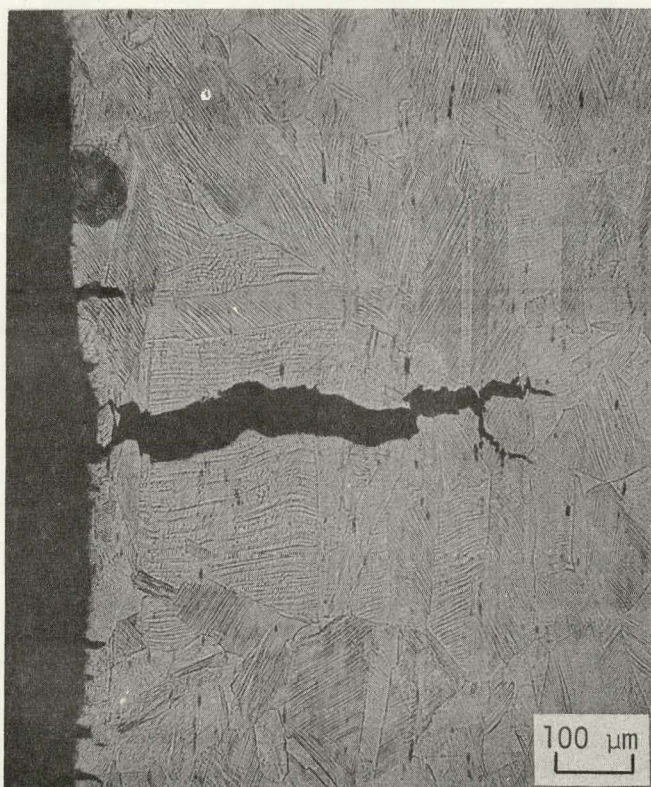
FIGURE 10. Surface Cracks of Deuterium-Saturated Specimen Tested at 273 K
