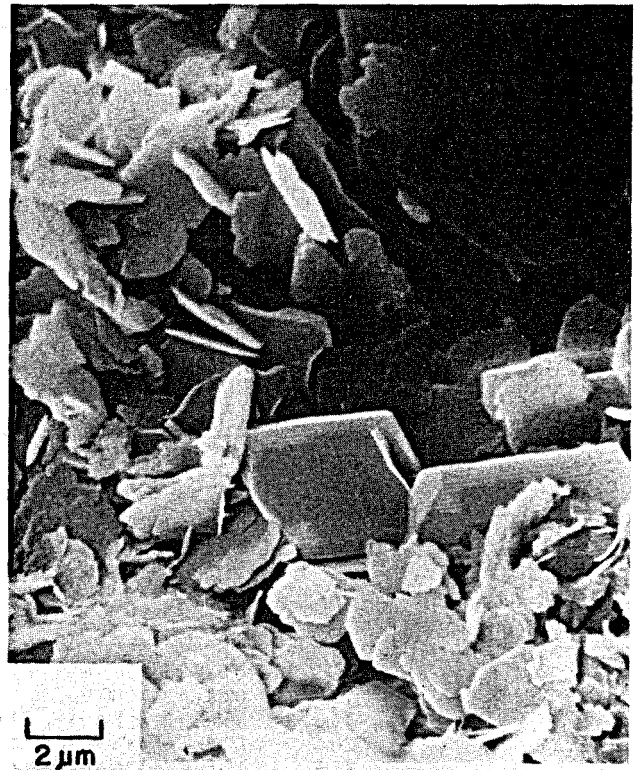
Figure 7. Authigenic muscovite plates and tubular orthoclase crystals in sandstone from 1274 m in Well M-26, Cerro Prieto. (Scanning electron micrograph.)
