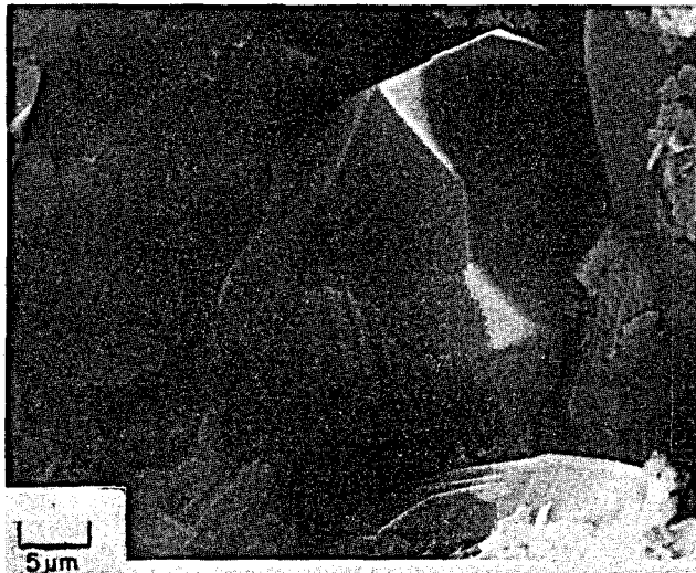
Figure 6. Authigenic equant wairakite crystal in sandstone from 1274 m in Well M-26, Cerro Prieto. The estimated original temperature of the sample is 305°C. (Scanning electron micrograph.)
