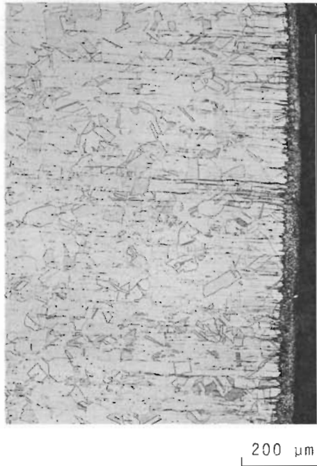
FIGURE 4. Optical Micrograph Showing the Disturbed Metal Layer at the Center of 0.6-cm Thick Stainless Steel Plate Cut Using a Plasma Torch
