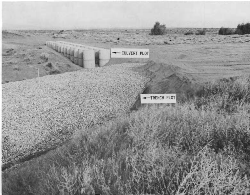
FIGURE 3. Location and Placement of Cobble Layer in the Trench Plot and the Arrangement of the Culvert Plot
