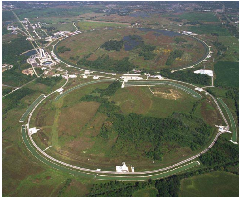
Figure 3.1: Aerial view of Fermilab showing the Main Injector in the foreground, the Tevatron collider ring and the fixed target facilities in the background.
