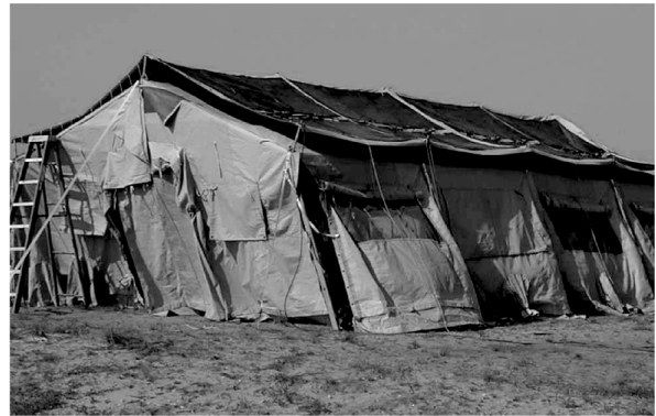
Fig. 10. Lightweight, flexible, thin-film CIGS modules deployed on U.S. Army tents.
