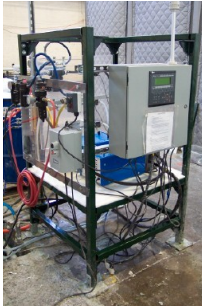
Figure 5: Error-proof Liquid Mixing System
