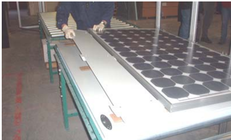
Figure 11: Completed Tile Assembly on the PL Factory Line
