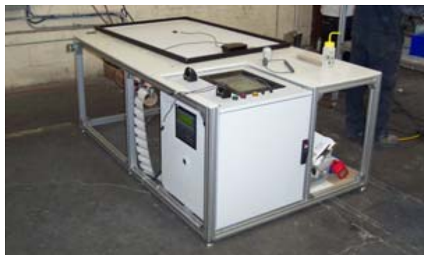
Figure 16: Dark I-V Module Test Station
