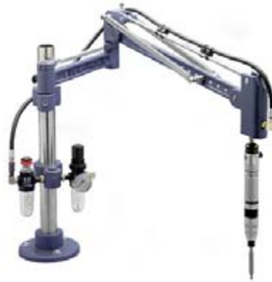
Figure 6: Proposed Pneumatic Screwdriver and Support
