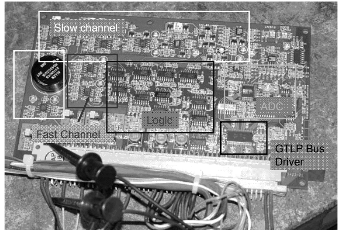
Fig. 3. Single channel PC board with different regions identified.
