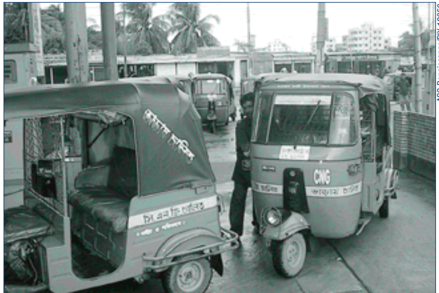
Thousands of three-wheel rickshaws in Dhaka have been switched from two-stroke gasoline power to four-stroke CNG fueling, and many more are slated for conversion in the future.
