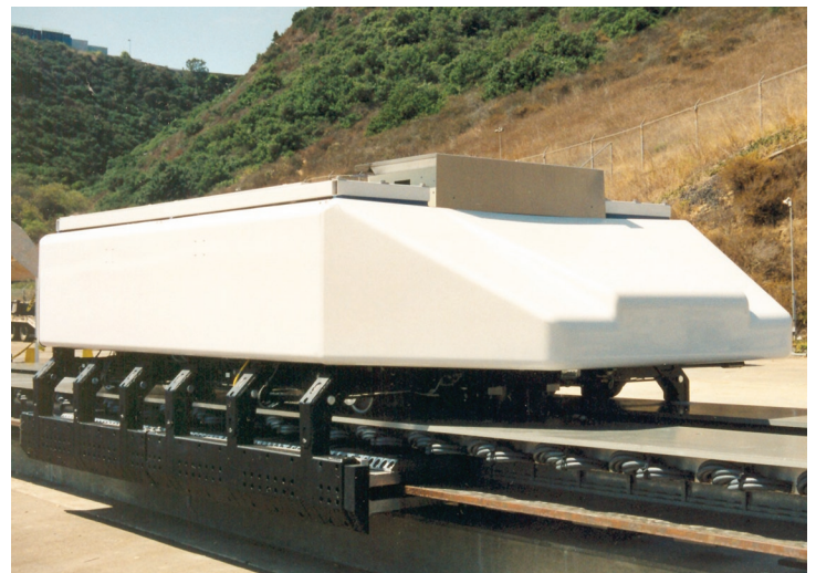
General Atomics' full-scale Inductrack test vehicle on the first section of the test track.
