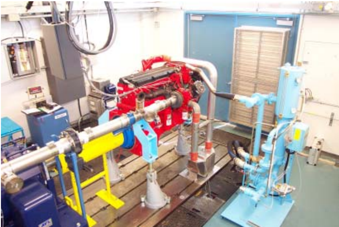
Figure 3: Test Cell with ISX Engine
