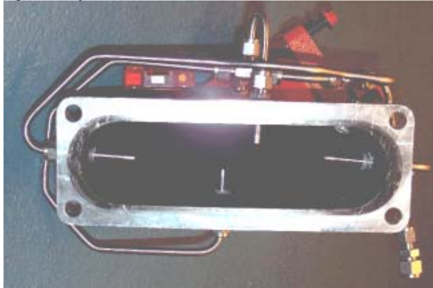
Figure 4: CO 2 Sampling Probes for Inlet Charge EGR Measurement
