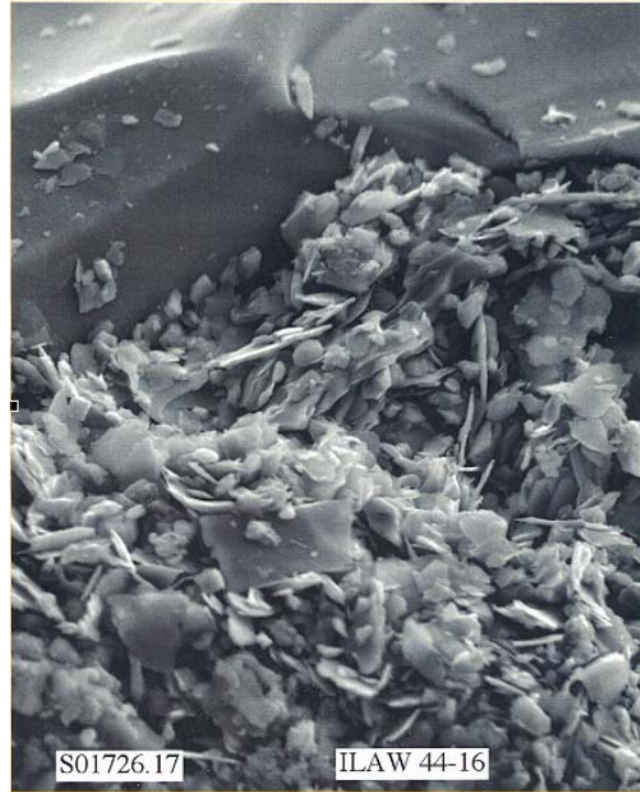
Figure 36. SEM Picture of Reacted Solids Removed From Static Corrosion Test with HSE Solution After 700 d at 40°C. Solids in the foreground are minerals extracted from Hanford Soil during preparation of the HSE solution.
