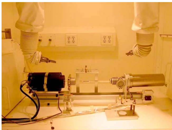
Figure C.19: Hot cell facility set-up(dilatometer) for post-irradiation CTE measurements.
