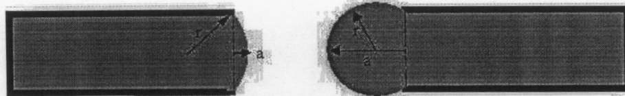
Figure 3.9: Radius, r , and injection length, a , of droplets before (left) and after (right) reaching a hemispherical shape where the radius is equivalent to the injection length.
