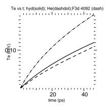
FIG. 2: The electron temperature as a function of time. The solid and dash-dot curves are the solution given in Eq. (5) for hydrogen and helium respectively with  $T_e(0) = .05 \text{eV}$ ,  $n_e = .007 n_c$ ,  $I = 1 \times 10^{14} \text{W/cm}^2$ , and laser wavelength,  $\lambda_0 = 1053 \text{nm}$ . The dashed curve is the pF3d solution with the strong field reduction.
