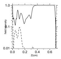
FIG. 4: The amplitude of  $A_0$  (solid) and the reflected light,  $A_r$  (dashed) at 23 ps with q=0.08 for an unheated hydrogen plasma. Other parameters are  $T_e = .05 \text{eV}$ ,  $n_e = .007 n_c$ ,  $I = 1 \times 10^{14} \text{W/cm}^2$ ,  $\lambda_0 = 1053 \text{nm}$ ,  $I_{\text{seed}} = 2.5 \times 10^{13} \text{W/cm}^2$ , and the initial seed pulse width,  $\tau = 40 \text{fs}$ .
