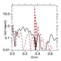
FIG. 5: The amplitude of  $A_0$  (solid black) and the reflected light,  $A_r$  (dashed red) of  $A_0$  at 35 ps with q=0.08 for an unheated hydrogen plasma. Other parameters are  $T_e = .05 \text{eV}$ ,  $n_e = .007 n_c$ ,  $I = 1 \times 10^{14} \text{W/cm}^2$ ,  $\lambda_0 = 1053 \text{nm}$ ,  $I_{\text{seed}} = 2.5 \times 10^{13} \text{W/cm}^2$ , and the initial seed pulse width,  $\tau = 40 \text{fs}$ .
