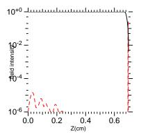
FIG. 6: The amplitude of the pump  $A_0$  (solid black) and the backscattered light  $A_r$  (dashed red) at 23 ps for a heated helium plasma with no pump chirp. Other parameters are  $T_e(0) = .05 \text{eV}$ ,  $n_e = .007 n_c$ ,  $I = 1 \times 10^{14} \text{W/cm}^2$ ,  $\lambda_0 = 1053 \text{nm}$ ,  $I_{\text{seed}} = 2.5 \times 10^{13} \text{W/cm}^2$ , and the initial seed pulse width,  $\tau = 40 \text{fs}$ .
