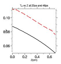
FIG. 3: The electron temperature (keV) is shown along the propagation direction at 23 ps when the seed is launched and at 46 ps when the amplified seed nears the boundary of the plasma at z=0. The simulation parameters are  $T_e(0) = .05 \text{eV}$ ,  $n_e = .007 n_c$ ,  $I = 1 \times 10^{14} \text{W/cm}^2$ , and pump laser wavelength,  $\lambda_0 = 1053 \text{nm}$ .
