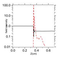
FIG. 7: The amplitude of the pump  $A_0$  (solid black) and the backscattered light  $A_r$  (dashed black) at 35 ps.for a heated helium plasma with no pump chirp. Other parameters are  $T_e(0) = .05 \text{eV}$ ,  $n_e = .007 n_c$ ,  $I = 1 \times 10^{14} \text{W/cm}^2$ ,  $\lambda_0 = 1053 \text{nm}$ ,  $I_{\text{seed}} = 2.5 \times 10^{13} \text{W/cm}^2$ , and the initial seed pulse width,  $\tau = 40 \text{fs}$ .
