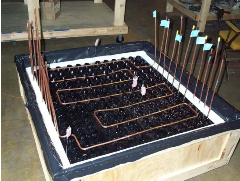
Figure 86. Heat storage module
