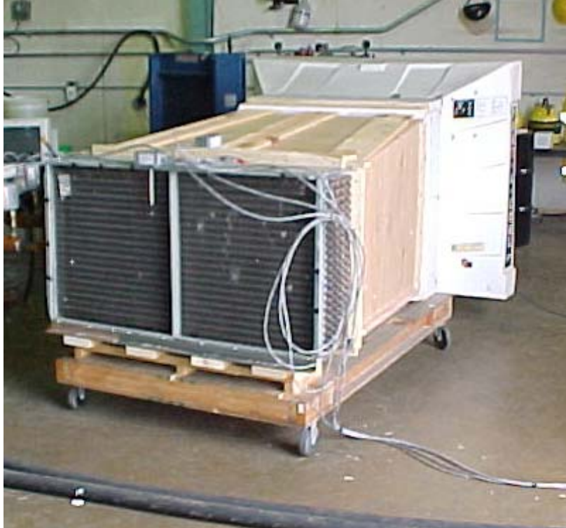
Figure 69. Cooling heat exchanger with instrumentation for warehouse
