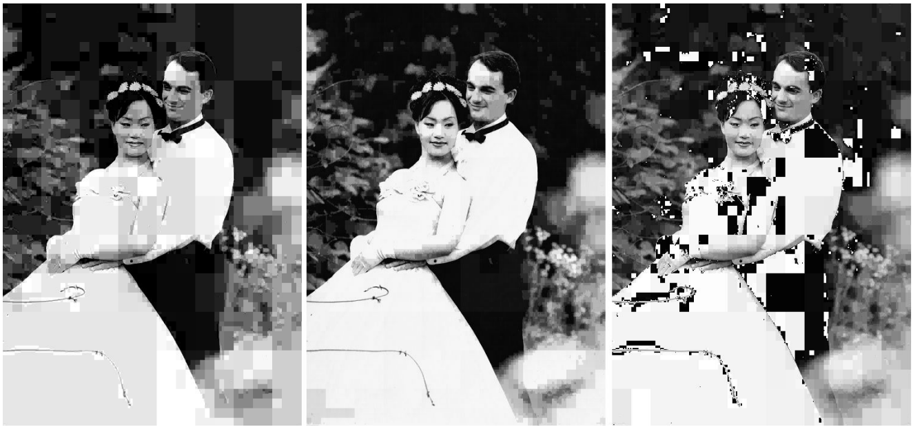
Figure 11. The Wedding photo, transformed (left to right) by the S, PLHaar, and CF transforms. Note the aliasing artifacts present in the CF reconstruction.
