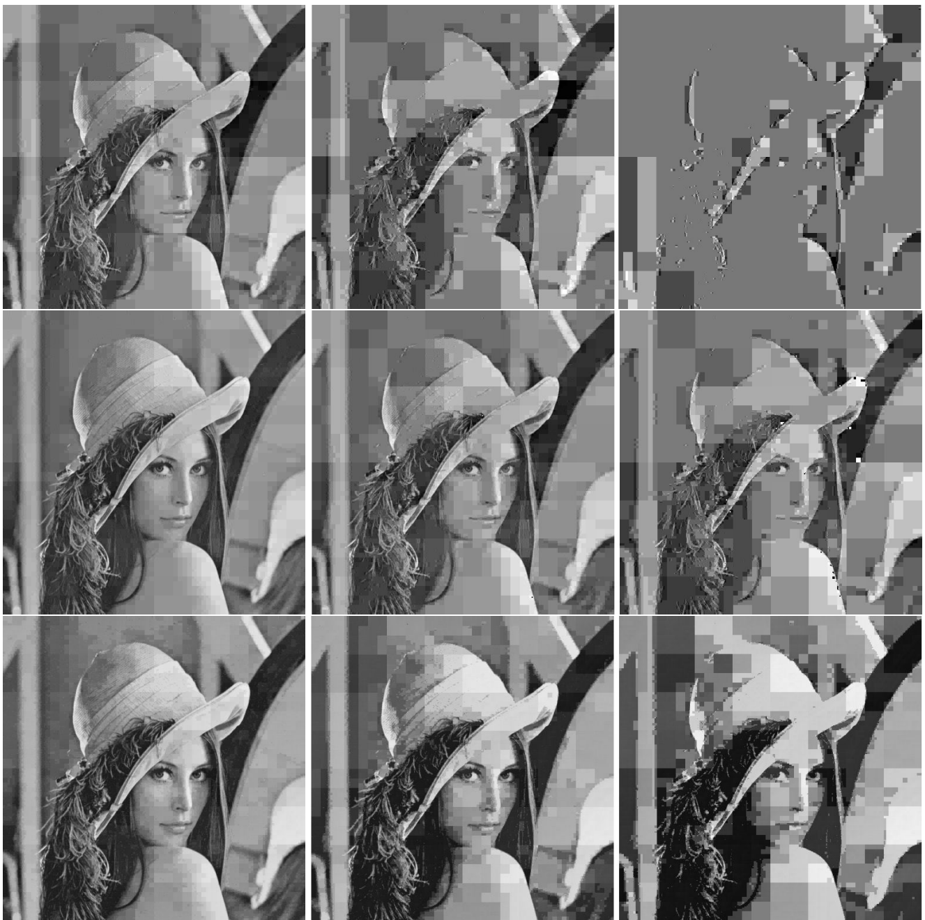
Figure 12. "Lena", with coefficients quantized to 5, 4, and 3 bits. From the top: S-Transform, CF, PL-Haar.
