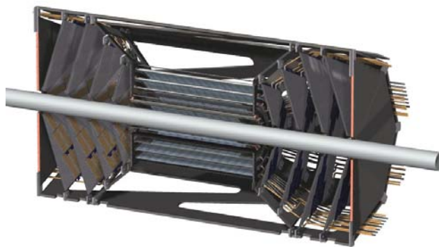
Figure 2. A schematic cut-away mechanical drawing of the proposed vertex detector (from Hytec).
