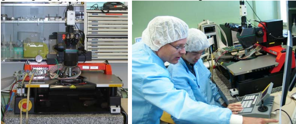
Figure 36 Left: Picture of the wafer probe station installed at CERN for the quality assurance tests of the pixel readout chips. Right: Quality assurance test of ALICE1LHCb readout chips in a clean room laboratory at CERN.
