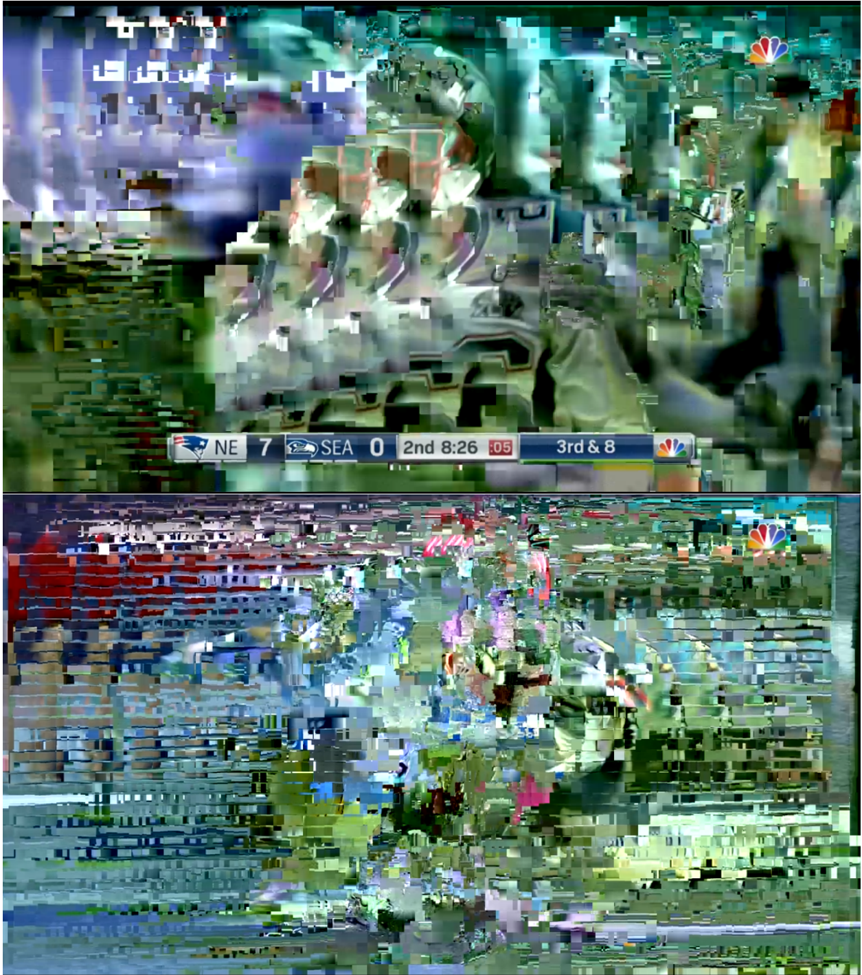
FIGURE 5.10. Screen shot of the video when the network is under attack. We can observe the video is completely distorted and the Quality of Experience (QoE) is very poor
