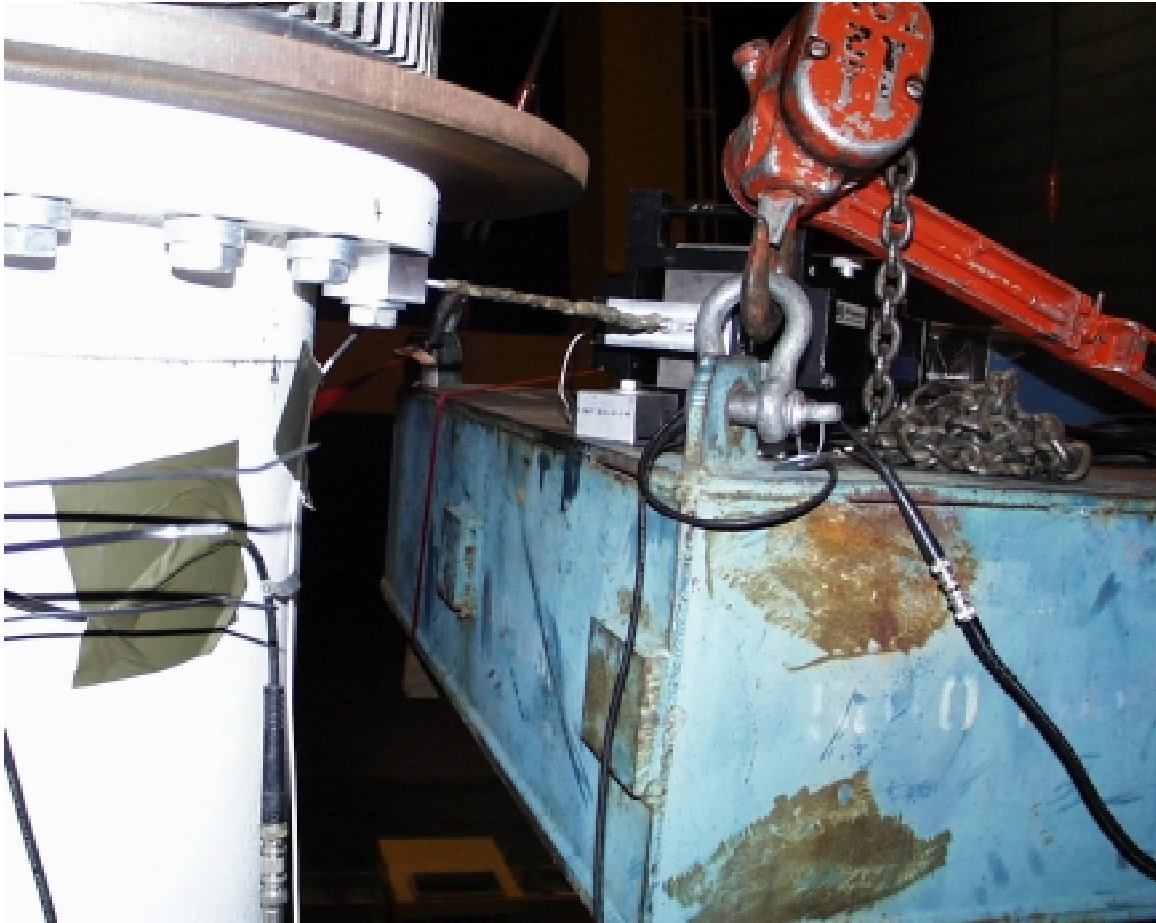
Figure A-19. Shaker mounted to steel reaction mass and attached to tower
