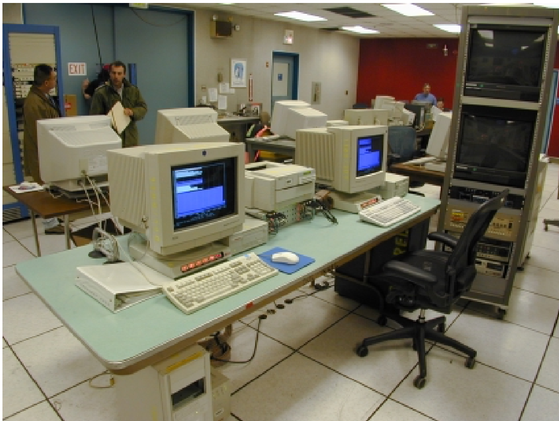
Figure 5. Wind tunnel control room. Data acquisition computer, turbine control computer, and video rack shown in foreground
