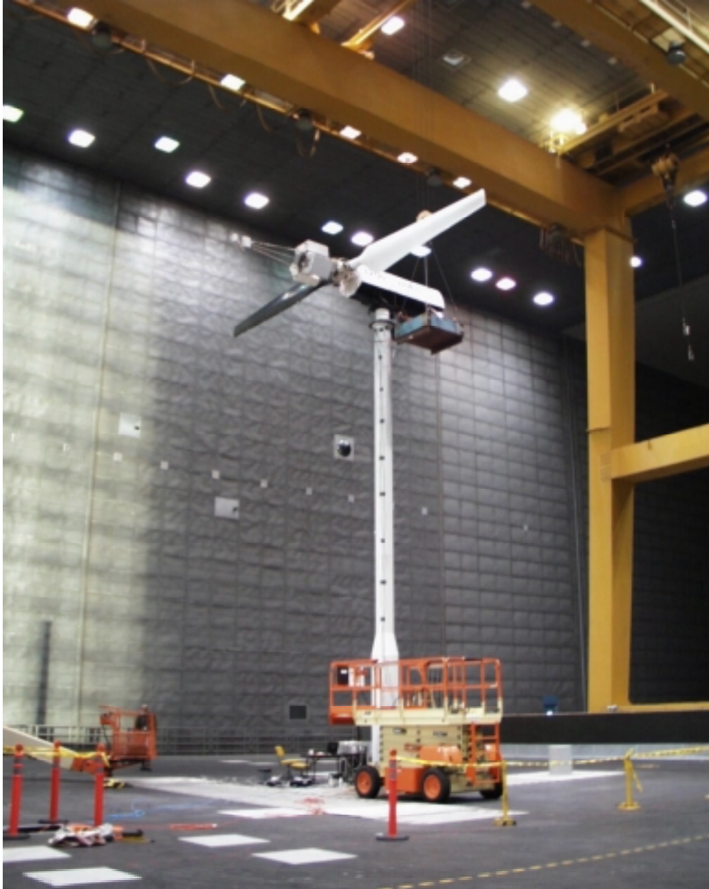
Figure A-18. Steel reaction mass suspended from gantry crane
