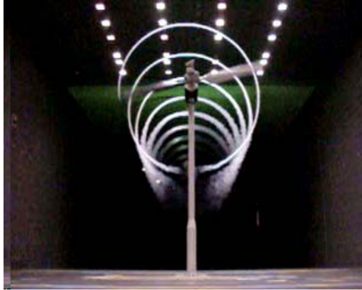
Figure J-2. Typical photo of wake flow visualization taken with digital still camera
