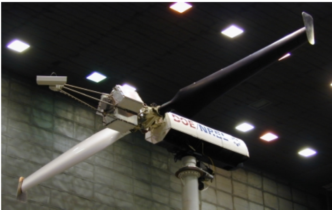
Figure A-8. Tip plates installed (Sequence V)
