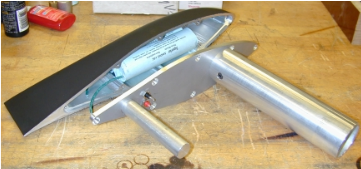
Figure A-5. Smoke tip with smoke generator inside
