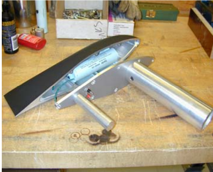
Figure J-1. Hollow aluminum blade tip with smoke generating cartridge installed
