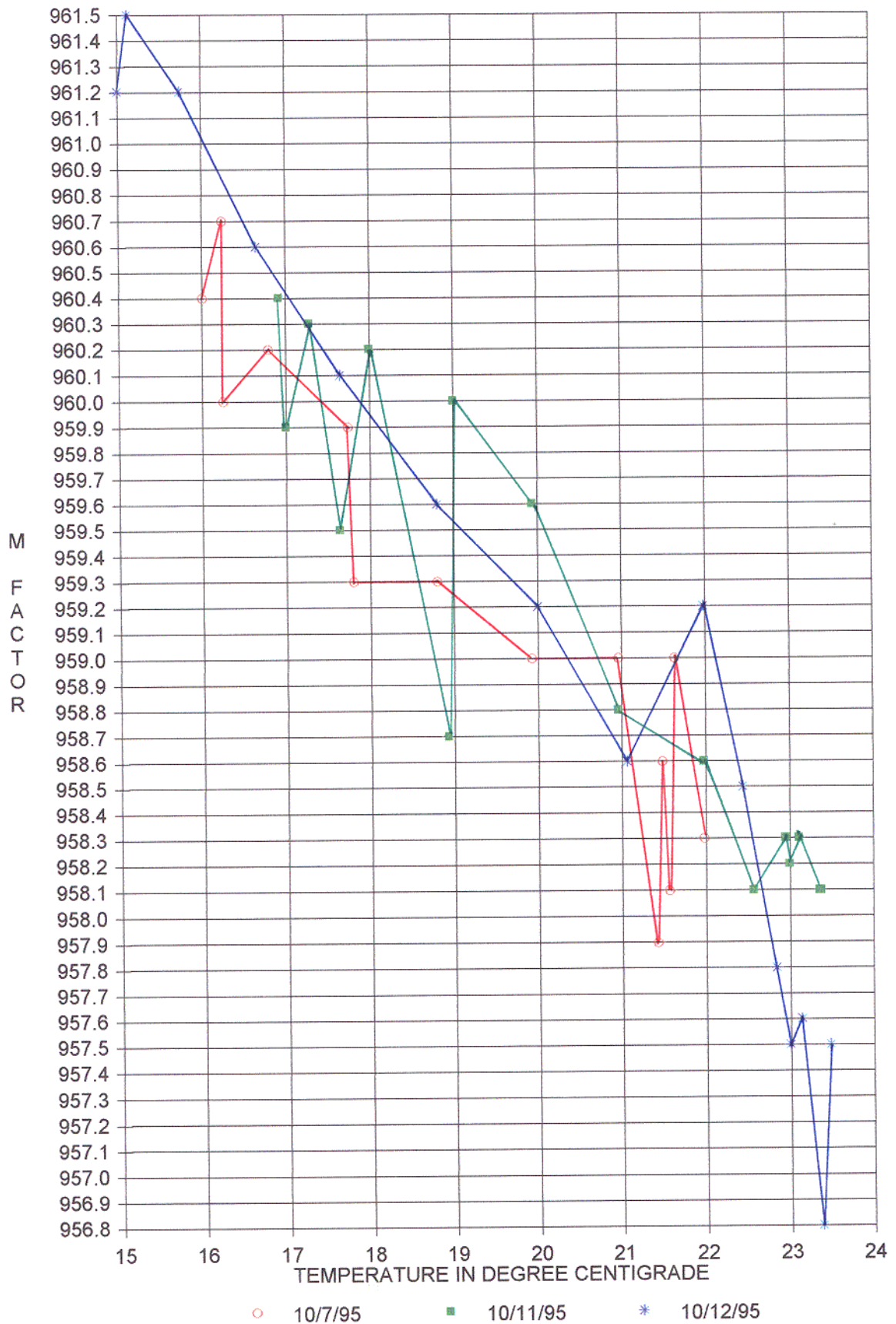
Fig. 8.10 Change of M Factor with Temperature for HF28968
