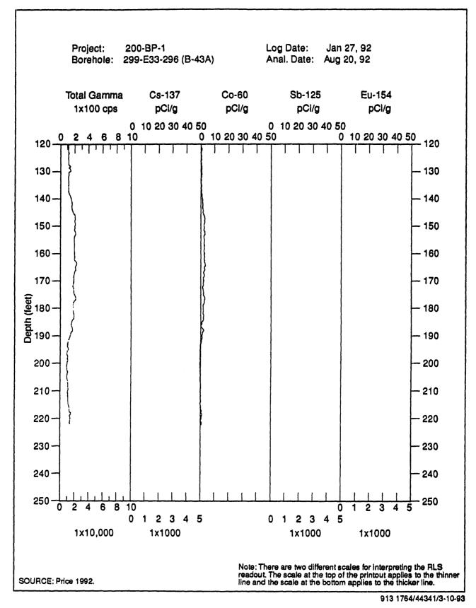
Figure 4-1b. RLS Spectral Gamma-Ray Survey of Borehole 299-E33-296 (216-B-43A). (Sheet 2 of 2)
