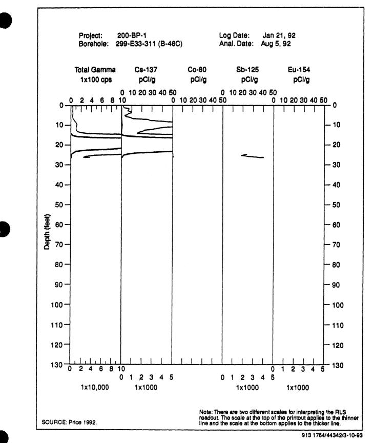
Figure 4-2. RLS Spectral Gamma-Ray Survey of Borehole 299-E33-311 (216-B-46C).
