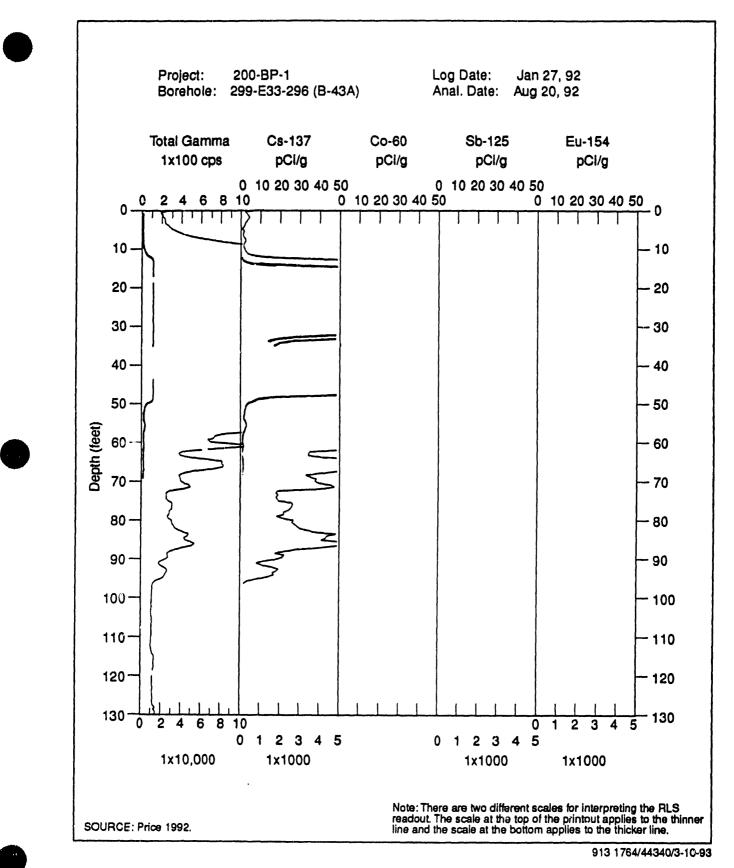
Figure 4-1a. RLS Spectral Gamma-Ray Survey of Borehole 299-E33-296 (216-B-43A). (Sheet 1 of 2)
