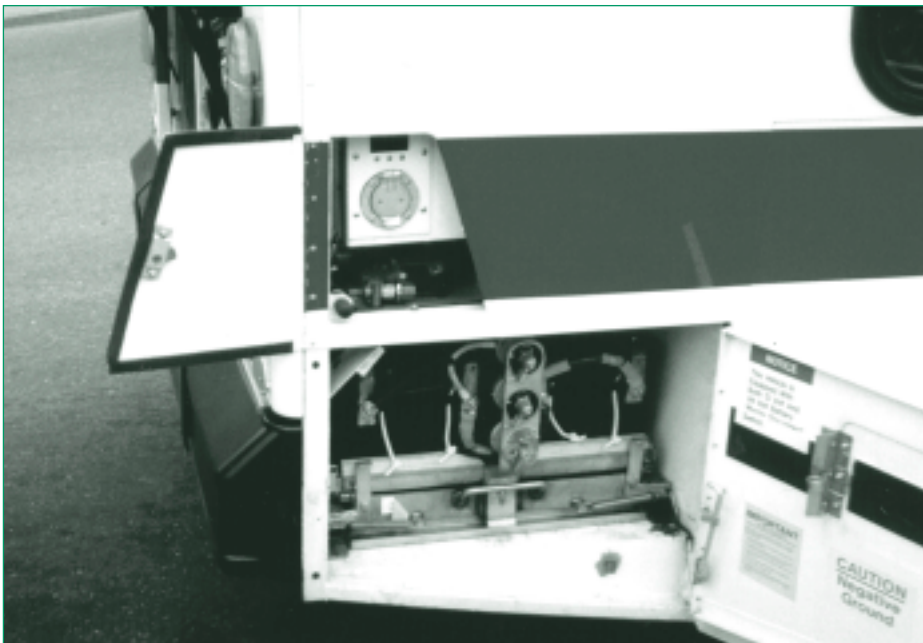
Figure 6. Rear quarter of hybrid bus showing battery conditioning port (top)
