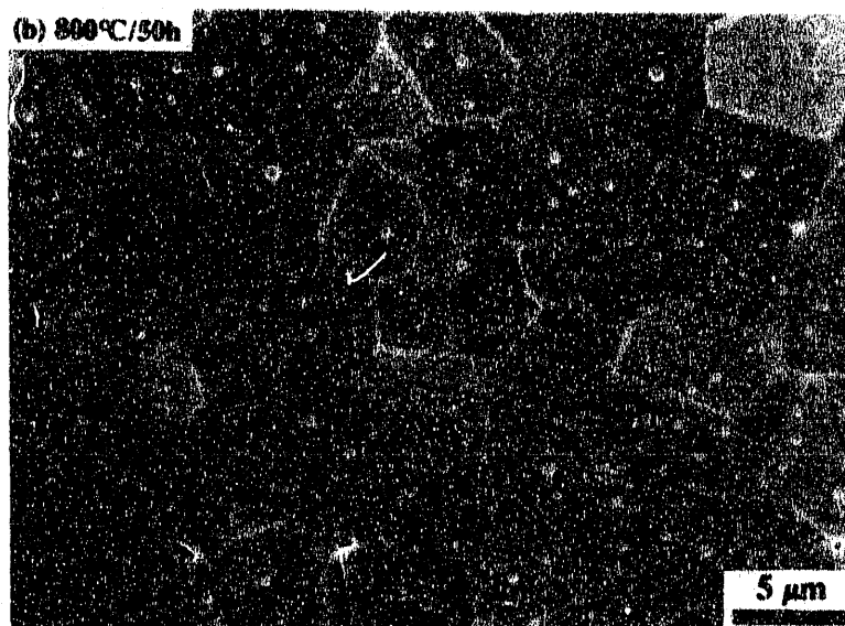
Figure 4.24 (Continued) Scanning electron micrographs of polished and thermally etched surfaces of MgO-doped \text{Al}_2\text{O}_3 samples fast fired in vacuum at a heating rate of 340^\circ\text{C}/\text{min.} to 1750^\circ\text{C} and held for 5 minutes: (a) conventional sample; (b) 800^\circ\text{C}/50 h homogenized; (c) 800^\circ\text{C}/100 h homogenized.
