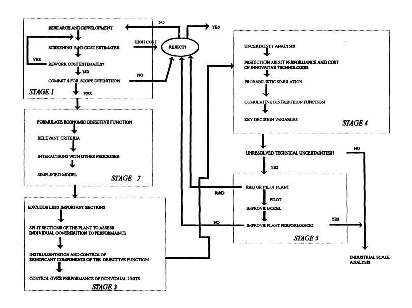
Fig. 2. Systems analysis methodology suggested to MWIP.
