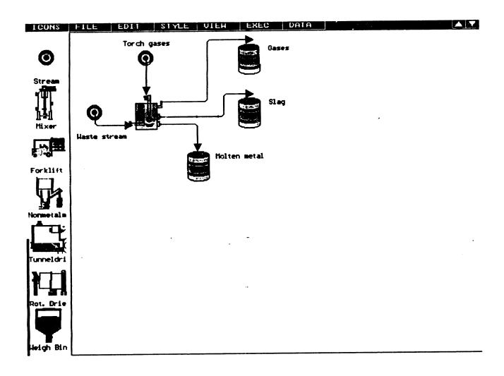
Fig. 5a. Graphical interface utilized by FLOW.
